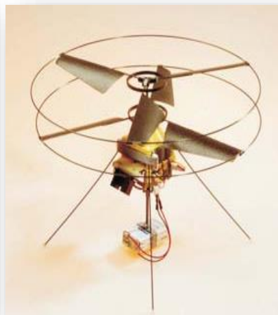
Figure I.6: Coax helicopter, developed at EPFL D'Ascanio Hélicoptère
