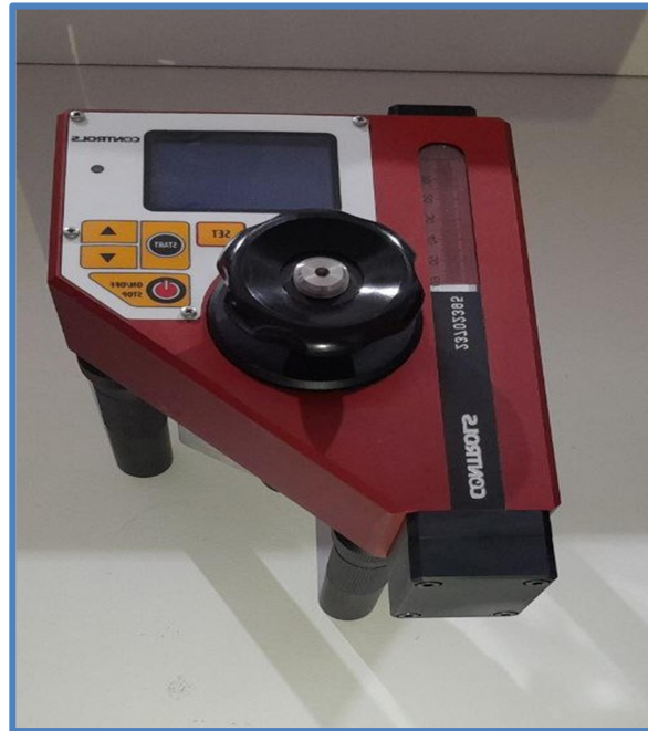
Figure (IV.24): Appareil utiliser pour l'essai d'arrachement (pull-off).
