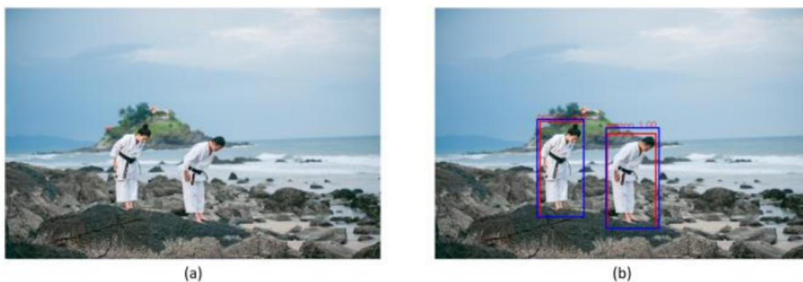
Figure 1.13: The sample shown in this section depicts, object detection with precise boundary boxes Blue and Brindha (2019).
