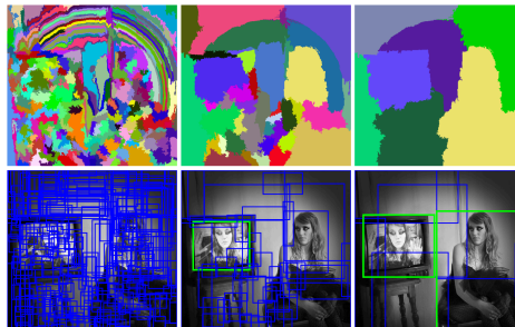
Figure 1.12: Hierarchical grouping algorithm finds objects at different scales, as the girl is contained by the TV van de Sande et al. (2011).
