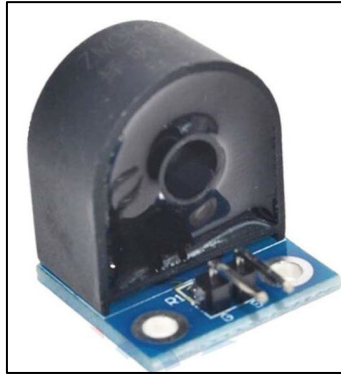
Figure 2.4: ZMCT103C Current sensor
