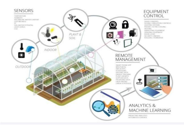
Find and compare available smart greenhouse monitoring systems. Monitor and control your entire operation remotely from your iPhone and Android device.
