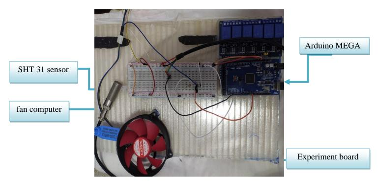
Figure III.3.2: Mounting the SHT 31 sensor
