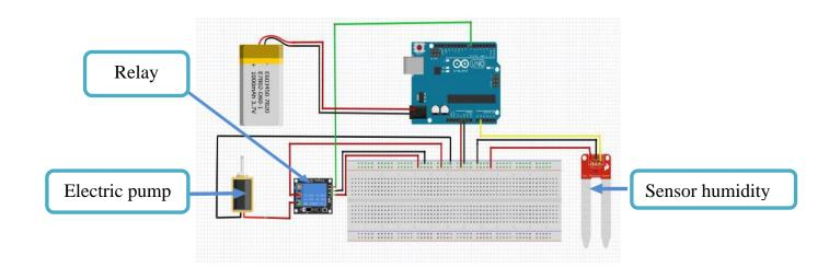
FigureIII.3.2: Mounting the soil moisture sensor.
