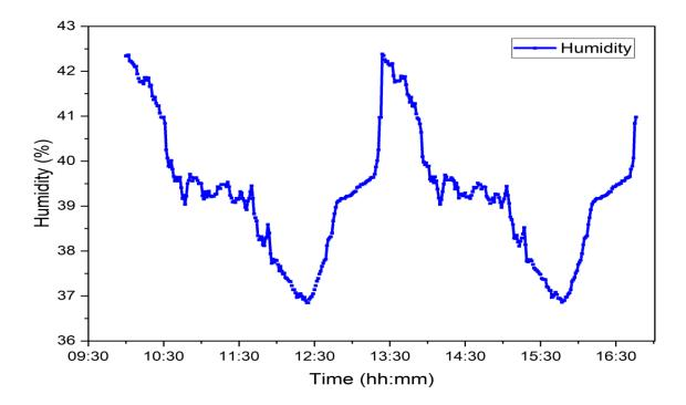
Figure (4): Humidity develops inside the greenhouse without control
