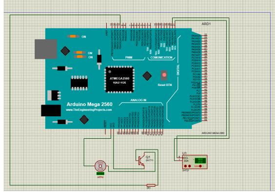
The schematic view of our service under the proteus software is shown in the figure III.3.2:
