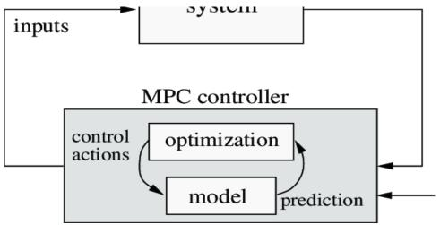
Figure (2): Illustration of model predictive control.
