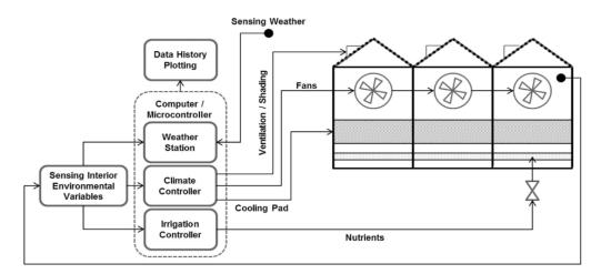
Figure I.8 Diagram of a Typical Hi-Tech Greenhouse [11].
