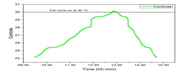
Figure (5): Temperature evolution in a greenhouse with control
