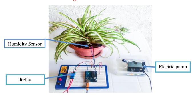
Figure III.3.1: Mounting the soil moisture sensor.
