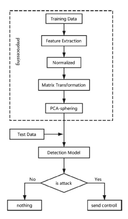
FIGURE 3.11 - Detection model by PCA-RNN [40]
