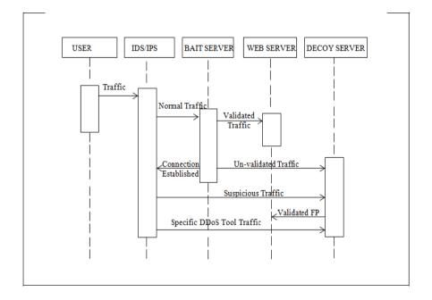
FIGURE 3.6 – Mitigation of DDoS attack traffic sequence. [48]
