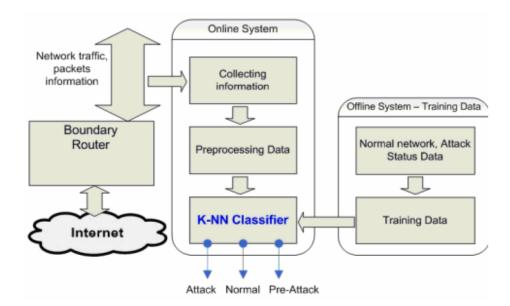
FIGURE 3.9 – General model for detecting precursor of DDoS attacks.[49]
