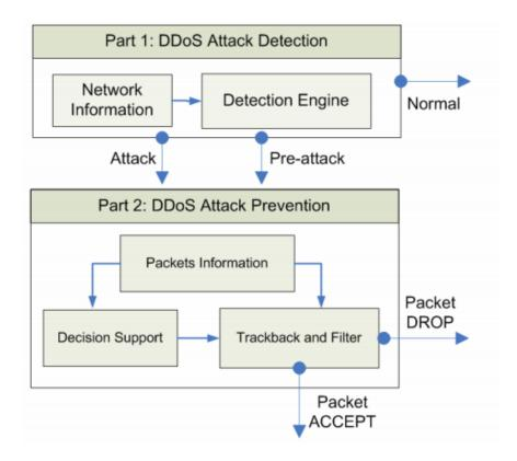
FIGURE 3.2 – A simple anti-DDoS framework[49]
