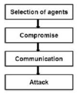
FIGURE 1.3 – Steps to perform a DDoS attack[10].
