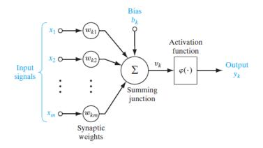
FIGURE 2.7 – Nonlinear model of a neuron, labeled k[27]
