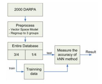
FIGURE 3.10 – Scheme of experiment [49]
