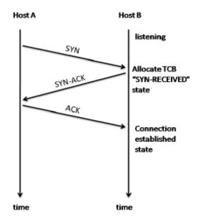
FIGURE 1.5 – TCP three-way handshaking [7].
