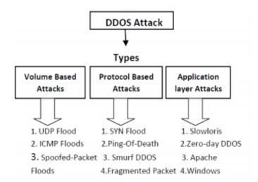
FIGURE 1.4 – Distributed DoS attack classification[42].
