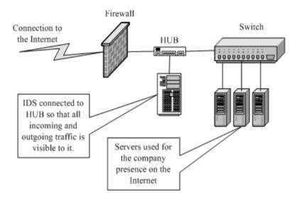
FIGURE 2.4: IDS connected in using hub [4].
