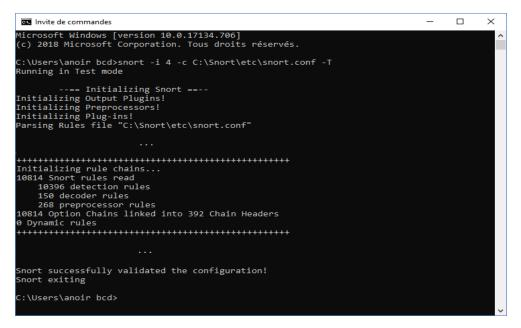
FIGURE 3.2: Test configuration file of Snort.
