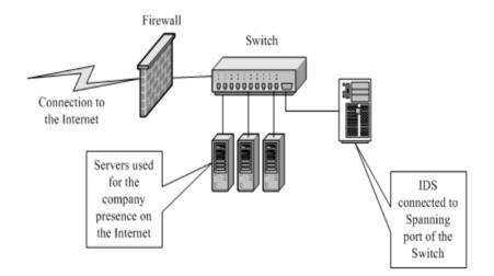
FIGURE 2.3: IDS connected in using switch [4].
