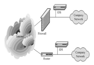
FIGURE 2.2: Typical locations for an intrusion detection system [4].
