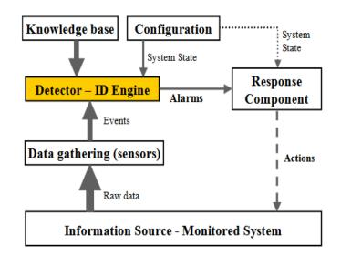
FIGURE 2.1: General architecture of an intrusion detection system [3].
