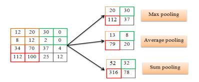
FIGURE 2.9: Pooling Layer
