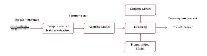
FIGURE 3.3: Automatic Speech Recognition Pipeline
