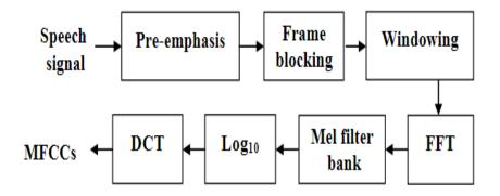
FIGURE 3.5: Steps of MFCC feature extraction
