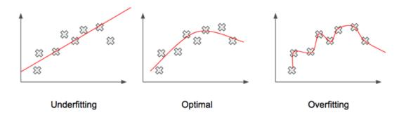
FIGURE 1.9: Over-fitting Problem, Optimal Case and under-fitting Problem
