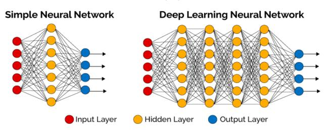
FIGURE 2.2: architecture of a simple neural network and deep neural network
