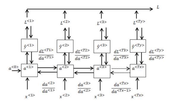
FIGURE 2.17: Backpropagation through Time
