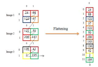
FIGURE 2.10: Flattening Layer
