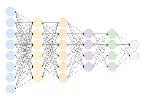
FIGURE 2.11: Fully Connected Layer
