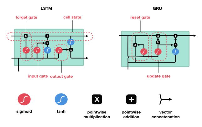
FIGURE 2.14: different between LSTM and GRU
