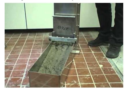
Figure (I.9) Procedure of L box test.
