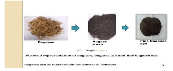
Figure (II.2) Stages access to Bagasse ash
