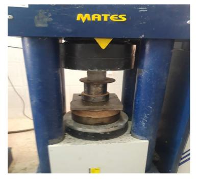
Figure (IV.1.) compressive strength machine.
