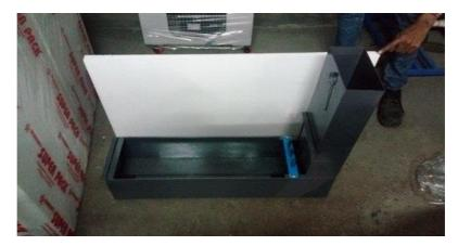
Figure (I.7) Equipment for L box test.
