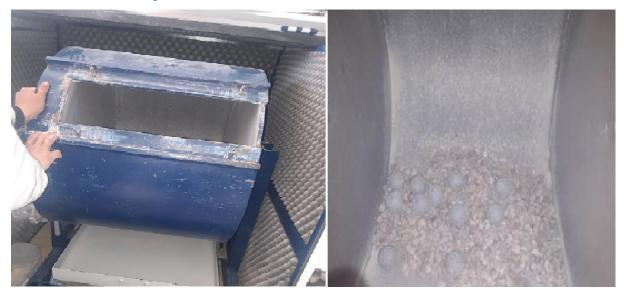
Figure (III.5)Los Angeles abrasion test
