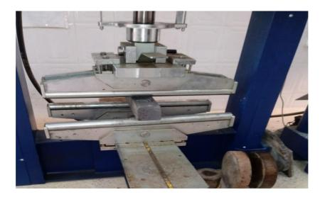
Figures (I.15) Bending tensile tests.
