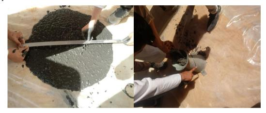
Figure III.8Slump Flow Test
