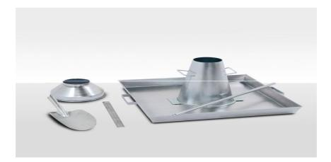
Figure (I.3) Equipment for slump flow test.
