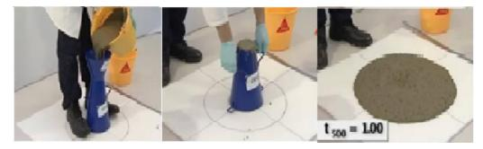
Figure (I.5) Procedure of slump flow test.
