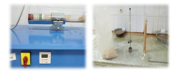
Fingure(III.3) The sand equivalent test.
