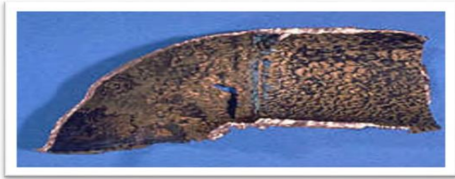
Figure N°I-4: Corrosion érosion /abrasion/cavitation
