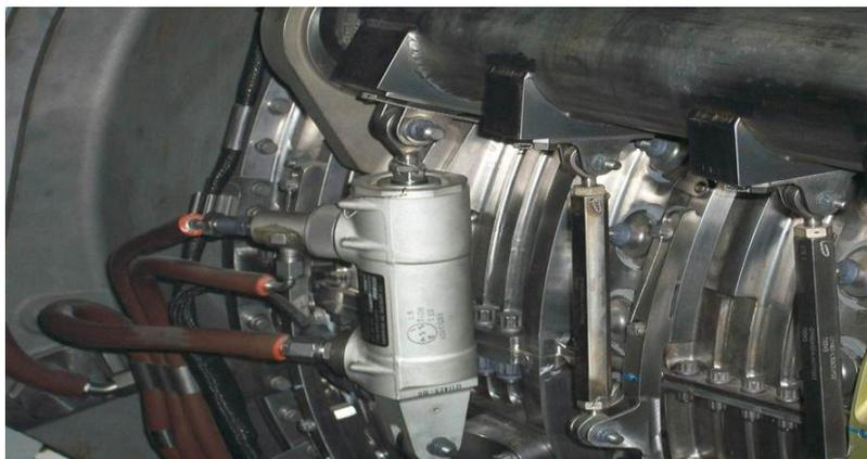
Figure III.13 :Vérin variable stator valve
