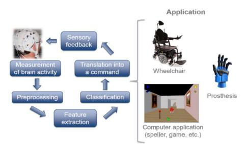
Figure 2. 6 : General architecture of brain-computer interface
