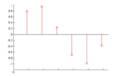
Figure 2. 9 : The sampling Continuous Signal into a Discrete
