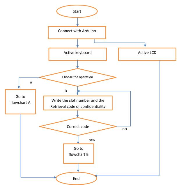
Figure II.5: Flowchart of keyboard using procedure.
