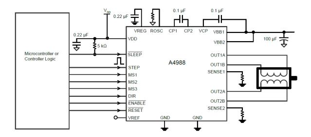
Figure II.8: Typical Application Diagram [35].
