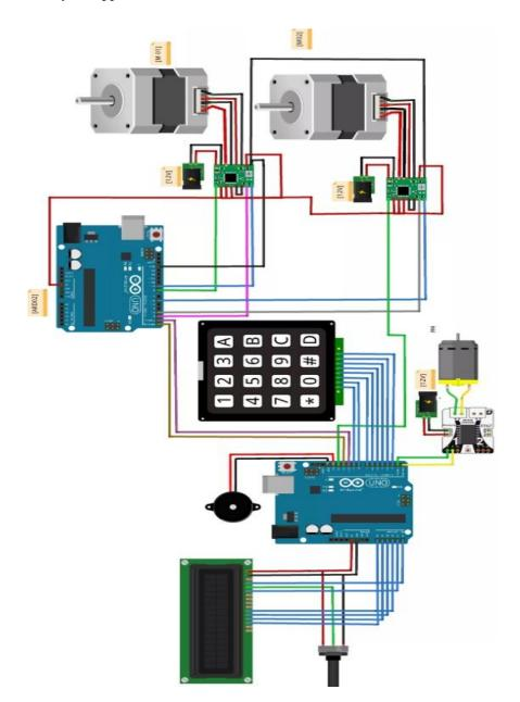
figure III.7: the electronic circuit designed using Fritzing.
