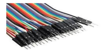
Picture II.12: DuPont Cable Wires [39].
