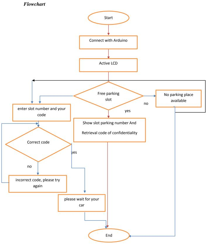
Figure II.2: Flowchart of display procedure.
