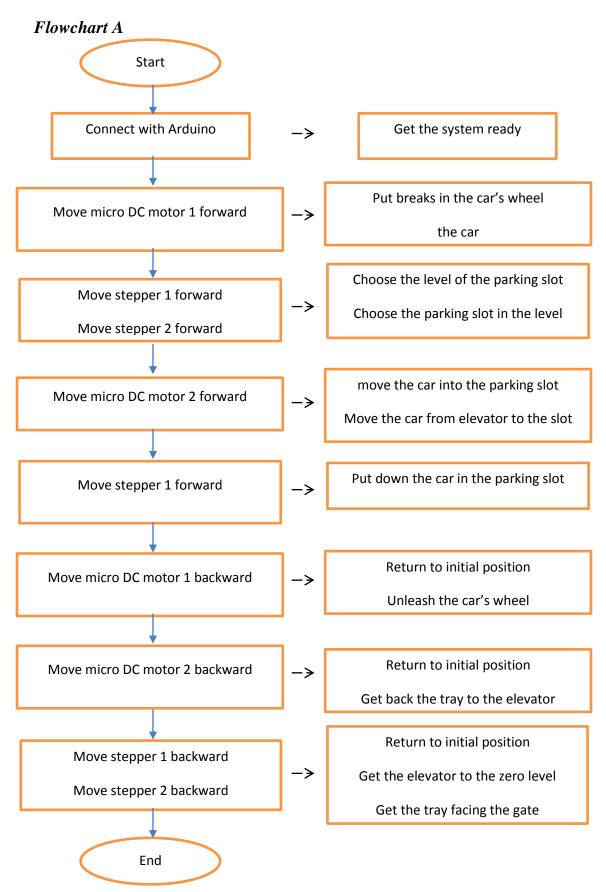
Figure II.6: Flowchart A of parking in procedure.
