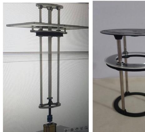
Figure III.4: the design the elevator.
