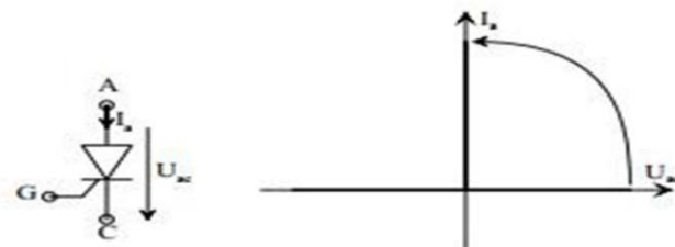
Figure I.2 : Thyristor symbol and switching .
