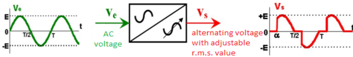
Figure I.8: dimmer's symbol and voltage input-output signal.[8]
