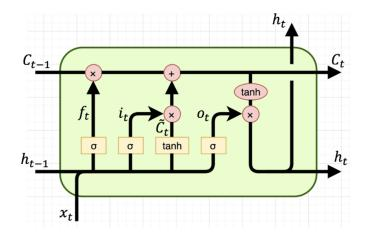
Figure 1.20: LSTM memory cell [10]
