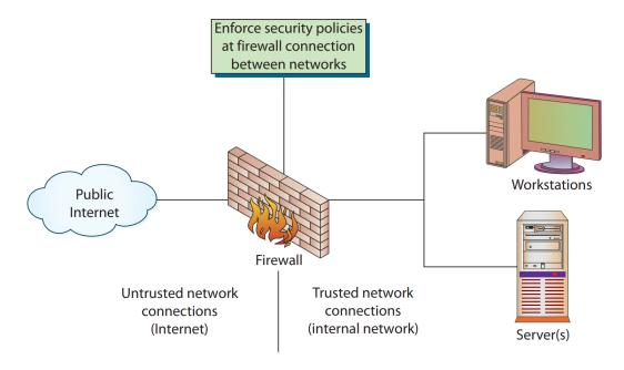
Figure 1.5: How a firewall works [9]
