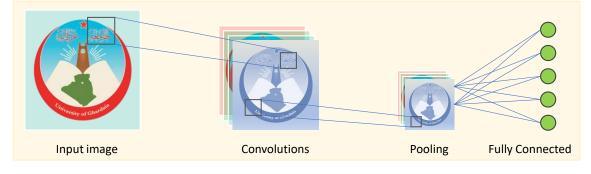
Figure 1.15: CNN Architecture
