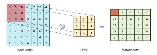
Figure 1.16: Convolution operation
