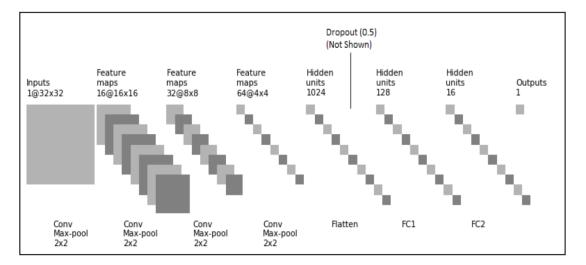
Figure 2.2: Deep Convolutional Neural Network (DCNN) for Intrusion Detection [13]
