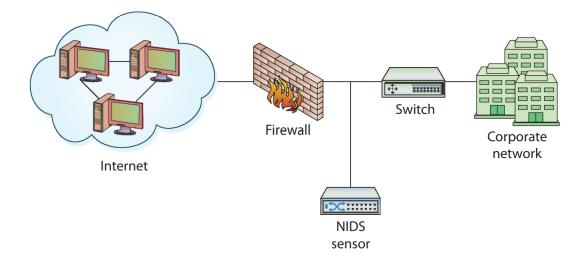
Figure 1.7: NIDS sensor placed behind firewall [9]
