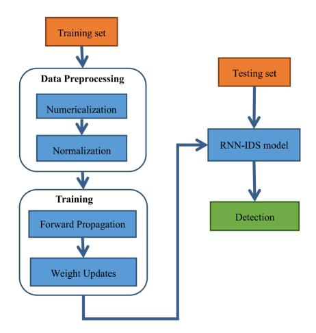
Figure 2.4: Block diagram of proposed RNN-IDS [56]
