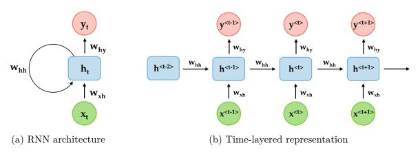
Figure 1.19: RNN architecture and it Time-layered representation [2]
