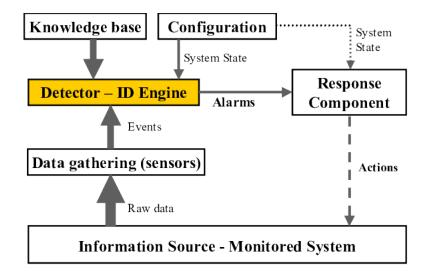
Figure 1.6: Basic architecture of an intrusion detection system (IDS) [41]
