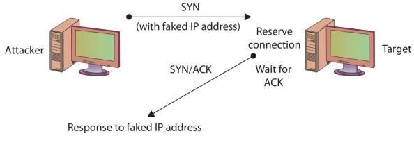
Figure 1.3: A SYN flooding based DoS attack [9]
