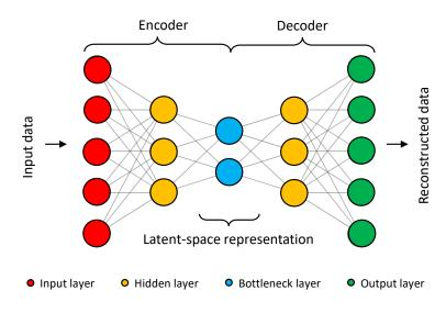
Figure 1.21: Autoencoder architecture
