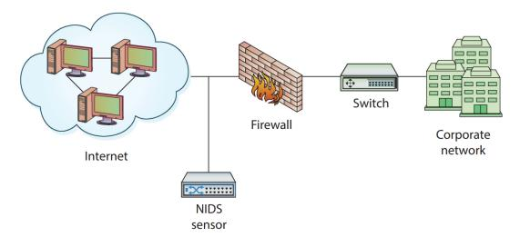
Figure 1.8: NIDS sensor placed in front of firewall [9]
