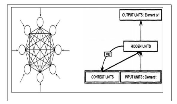
Figure 5 The architecture of a Recurrent Neural Network.
