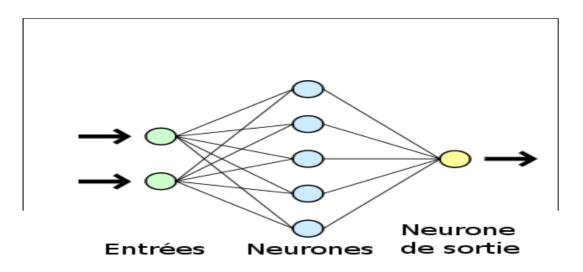
Figure 3. The architecture of a simple perceptron
