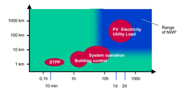
Fig. 5: Typical target applications for irradiance forecasting and their respective spatial and temporal scales. (STPP = Solar Thermal Power Plants, PV = Photovoltaics). The blue area depicts the range for which the use of Numerical Weather Prediction models is appropriate.
