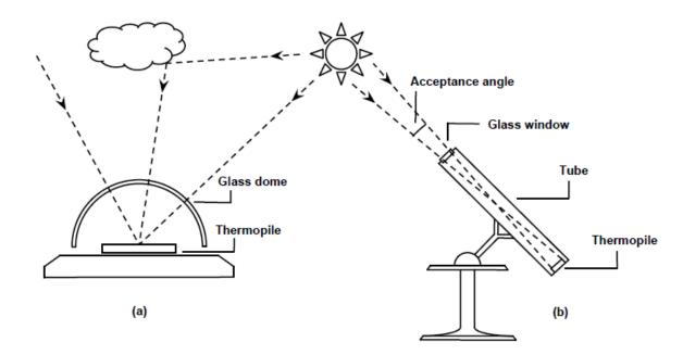
Fig 4: A schematic illustration of a pyranometer (a) and a pyrheliometer (b)
