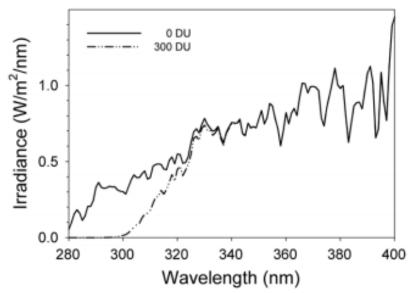
Fig1: Illustration of the effect of ozone on spectral surface UV irradiances
