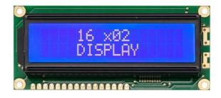
FIg 22: 16x2 LCD screen
