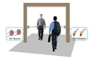
FIg 7: LDR and Laser diode solution
