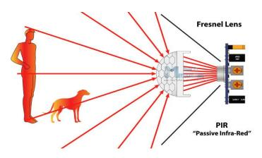
FIg 5: infrared motion sensor
