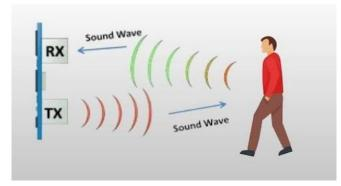
FIg 3: ultrasonic Sensor
