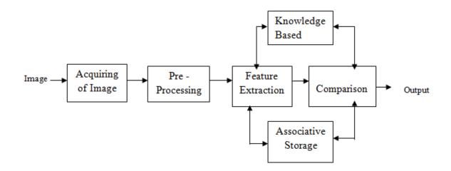
FIg 13: Digital image processing system
