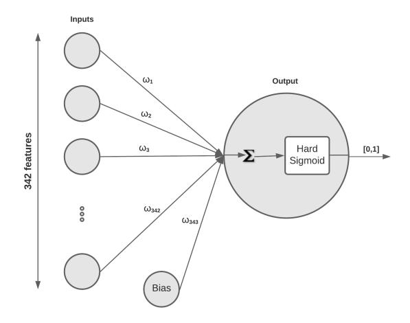
Figure 4.2: Proposed method using the Preceptron model diagram
