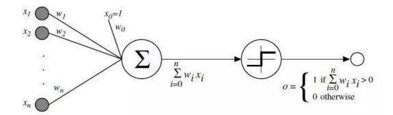
Figure 4.1: A diagram showing how the Perceptron works [77]
