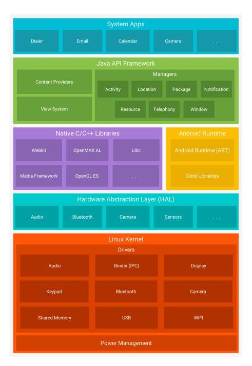
Figure 1.1: Android platform architecture [3]
