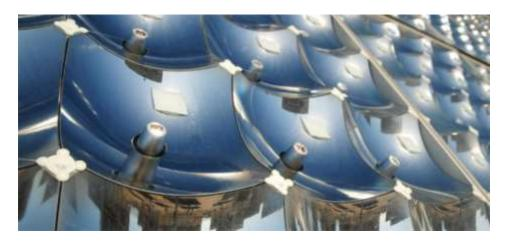
Figure 26 : The concentrated photovoltaic
