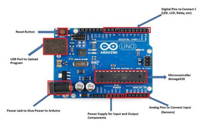
Figure III-1: Diagram of Arduino Uno [17].
