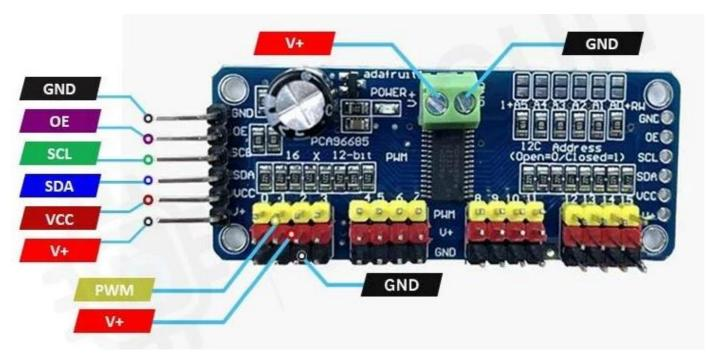
Figure III-12: Driver Motor PCA9685 [31].
