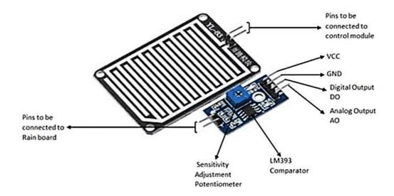
Figure III-3: Yl-83 Rain Detector [22].
