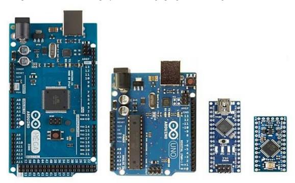
Figure II-3: Types of Arduino Boards [17].
