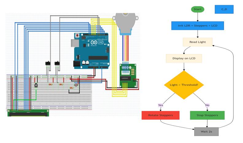
Figure IV-9: Wiring diagram [43].
