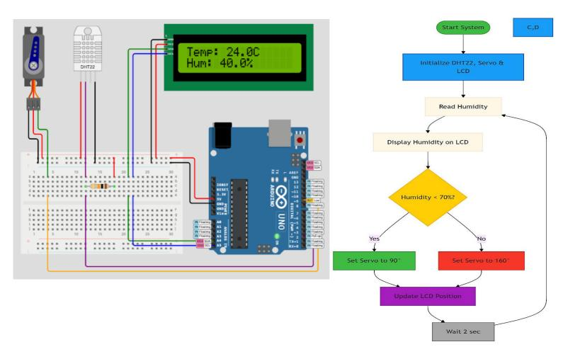
**Figure IV-3:** Wiring diagram [40].
