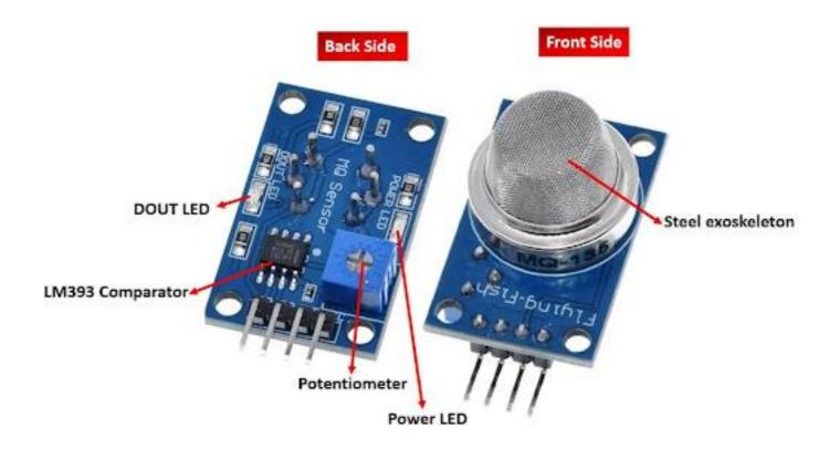
Figure III-5: MQ-135 Sensor [24].
