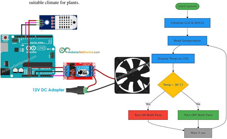
**Figure IV-1:** Wiring diagram [39].
