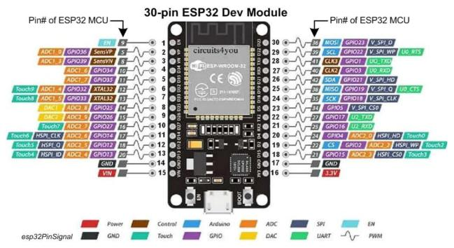
Figure III-16: ESP32 Datasheet [34].
