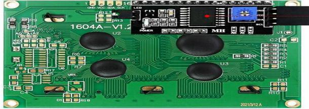
**Figure III-8:** LCD I2C 16×4 [27].
