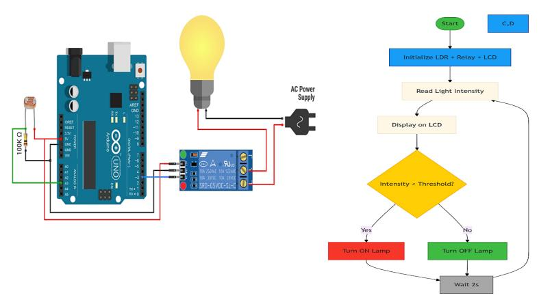
Figure IV-7: Wiring diagram [42].
