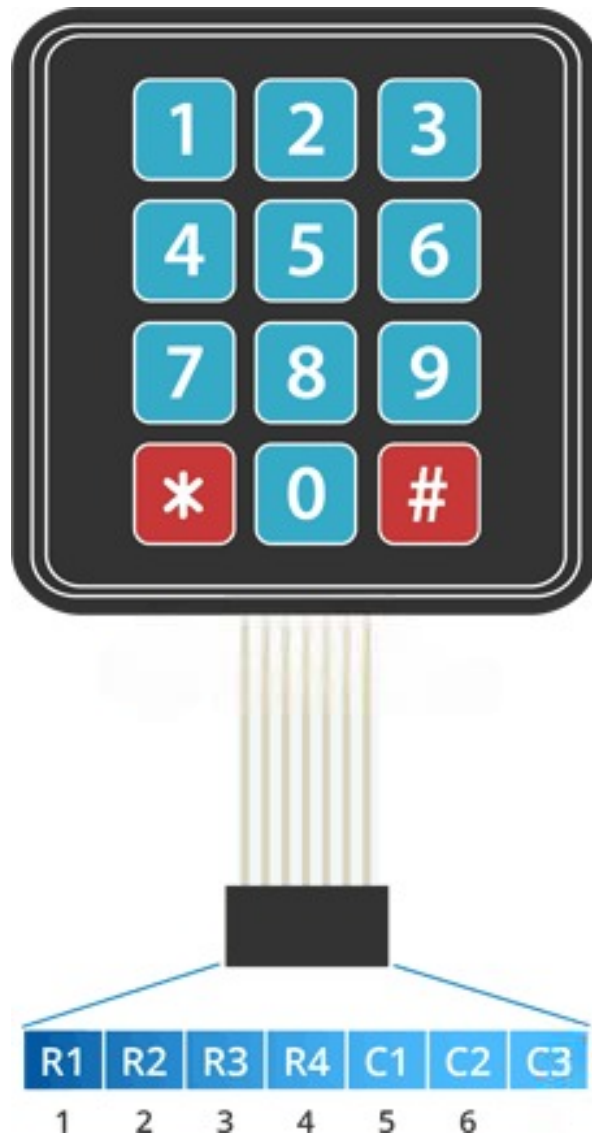
Figure 3.8: 4x3 Membrane Keypad Pinout
