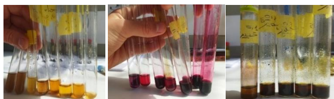
Figure. III.18: DPPH Test for the extracts
