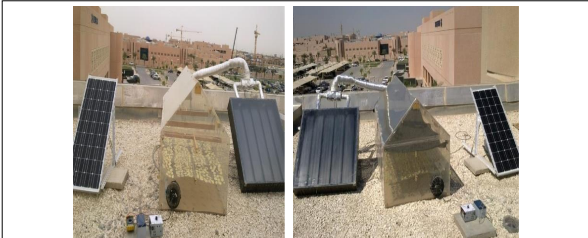
Figure II. 29: Experimental setup of solar PV powered enhanced tunnel dryer for potato chips. a) Without shading the potato chips, b) with shading the potato chips (black thermal curtain).
