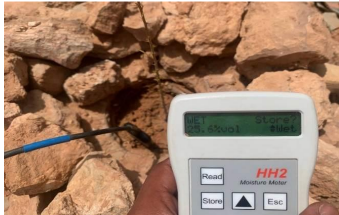
Figure 7: Humidity value on the device after first week watering
