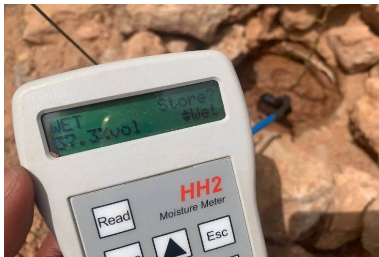
Figure 4: The humidity value on the device for the first time watering the tree with the cocoon
