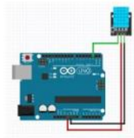
Figure 3-5 : Wiring of a DHT11 sensor on the Arduino Uno
