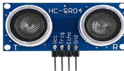
Figure 2-11 HC-SR04 ultrasonic sensor [17]
