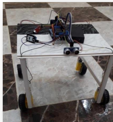
Figure 3-1 AGROBOT mobile robot in the early development stage
