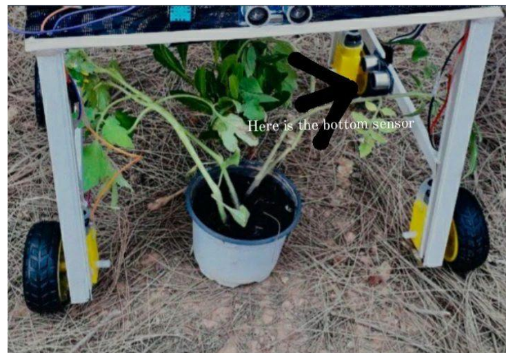
Figure 3-10 The bottom sensor for plant detection
