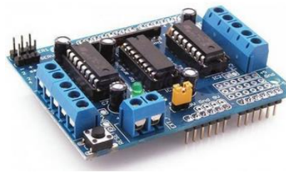
Figure 2-21 L293D Motor Driver Shield [26]
