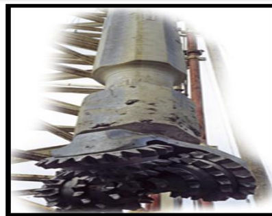
Figure 3-01 : La sonde de forage Rotary.
