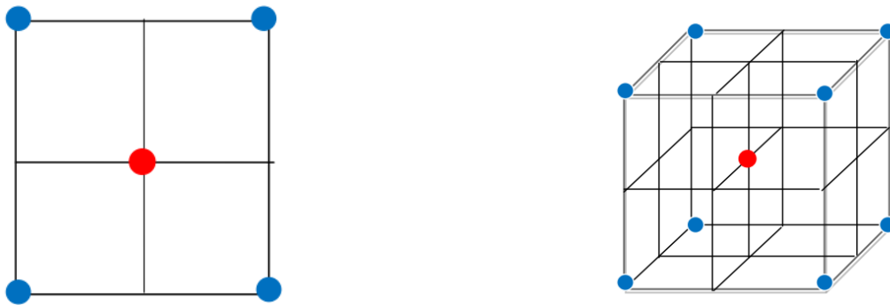
Figure1. 10: in the right Two-level full factorial design for two factors, in the left Two-level full factorial design for three factors. [11]
