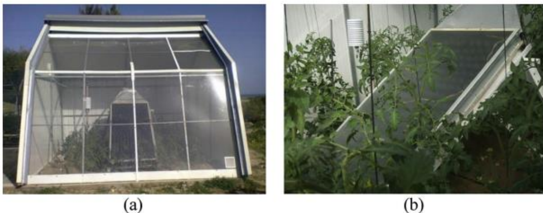
Figure II-8: a) External view of the insulated greenhouse, b) Solar air heater with LTES inside the greenhouse [43]
