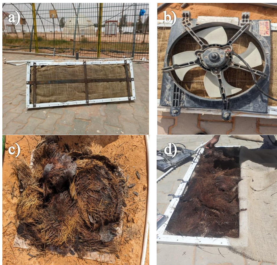
Figure III-22: components of Fan-Pad cooling system: a) Evaporative cooling pad, b) Fan, c) Palm leaf, d) Arranging palm leaf inside an evaporative cooling pad.
