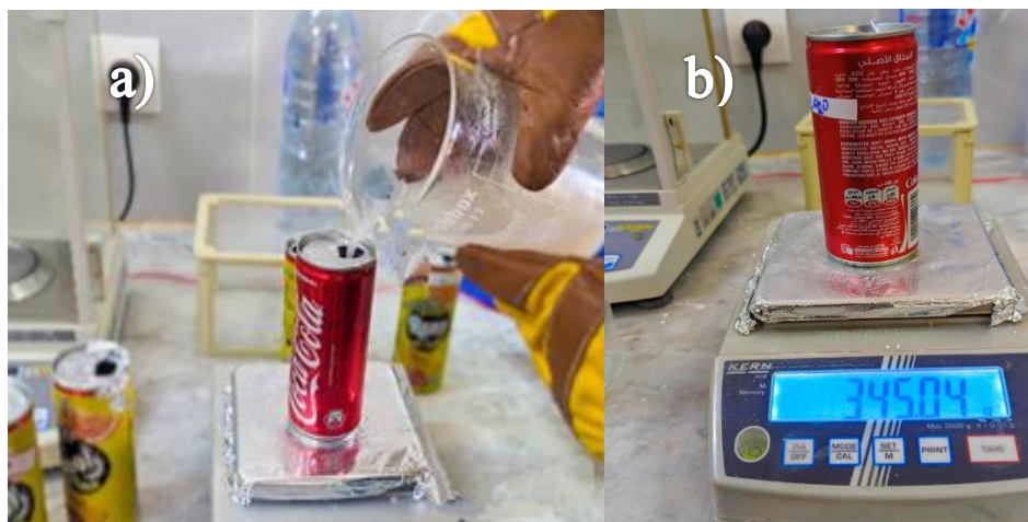
Figure III-13: a) Pouring the mixture of hydrated calcium chloride into the cans.
