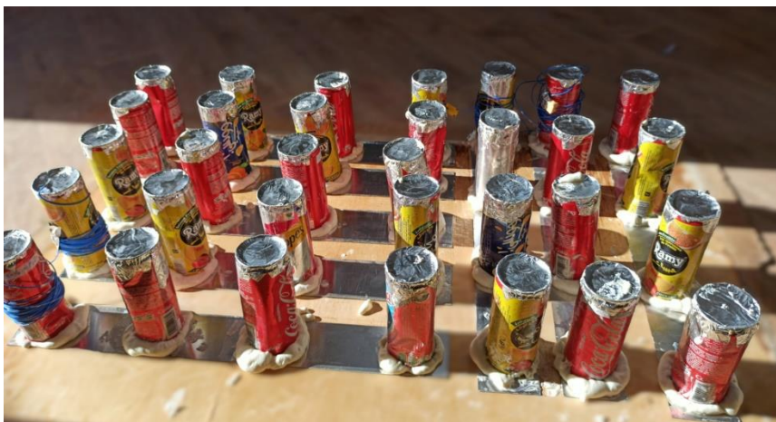
Figure III-11: Cans of chloride calcium \text{CaCl}_2, 6\text{H}_2\text{O}
