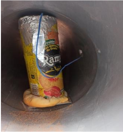
Figure III-6: Disposition PCM cans
