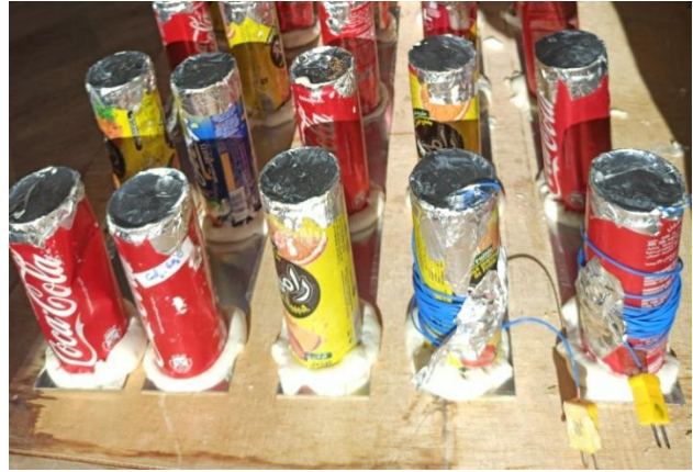
Figure III-7: PCM cans with a diameter of 60mm
