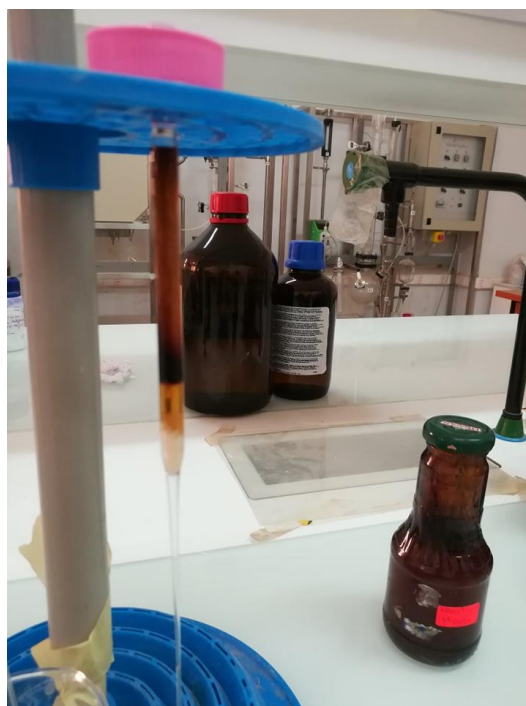
Figure 22: Chromatographie sur colonne de Gatran Djelfa
