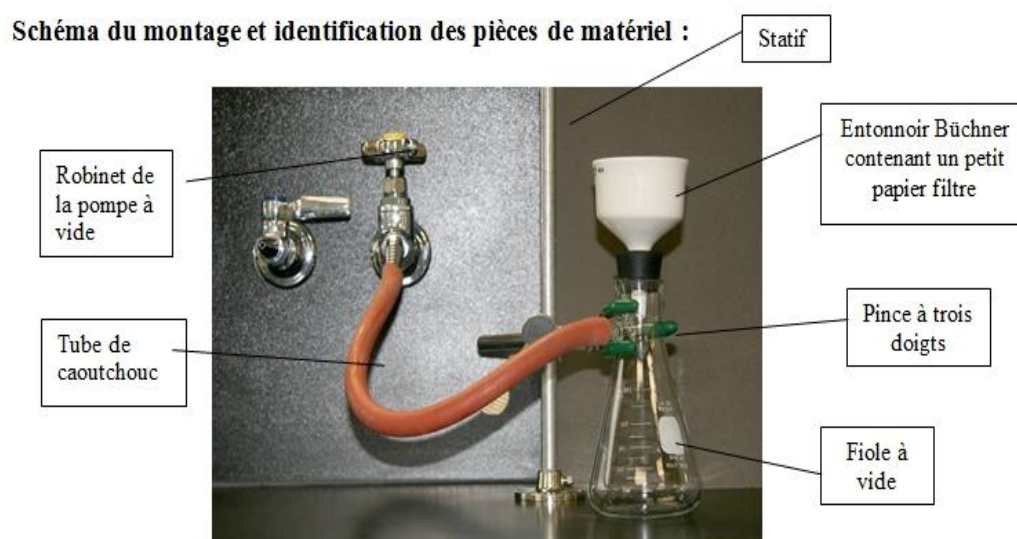
Figure 20: Filtration sous vide [33].
