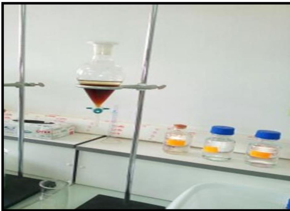
**Figure 14** : Extraction liquide- liquide (origine).
