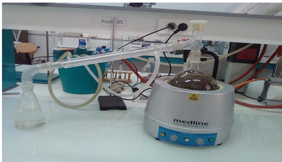
**Figure III.5:** Montage de distillation A.E (2018)
