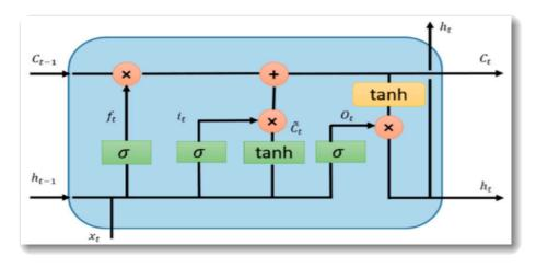
Figure 2.23: LSTM cell
