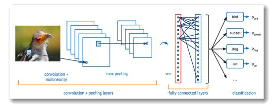
Figure 2.15: CNN Architecture
