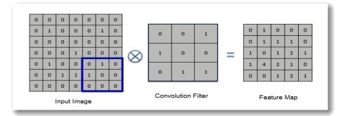
Figure 2.16: Convolution operation
