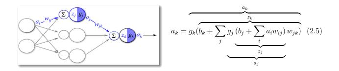
Figure 2.7: Forward-propagate
