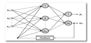
Figure 2.6: Feedback architecture
