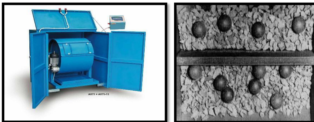
Figure .III.6: Essai de LOS ANGLES
