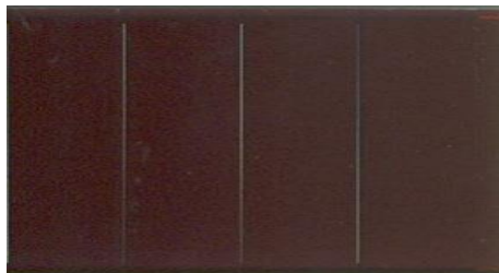
Figure I. 9 : Cellule photovoltaïque amorphe [01]
