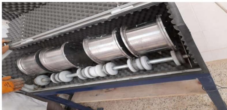
**Photo .II.15. La Machine Micro Duval**
