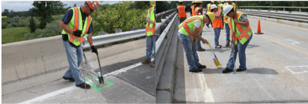
Figure 1.2: Hammer sounding and chain-drag testing [1].
