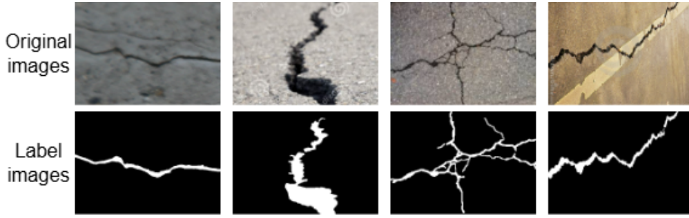
Figure 3.1: The first row is the original image which is the DeepCrack data set, and the second row is the artificial mark of the crack.
