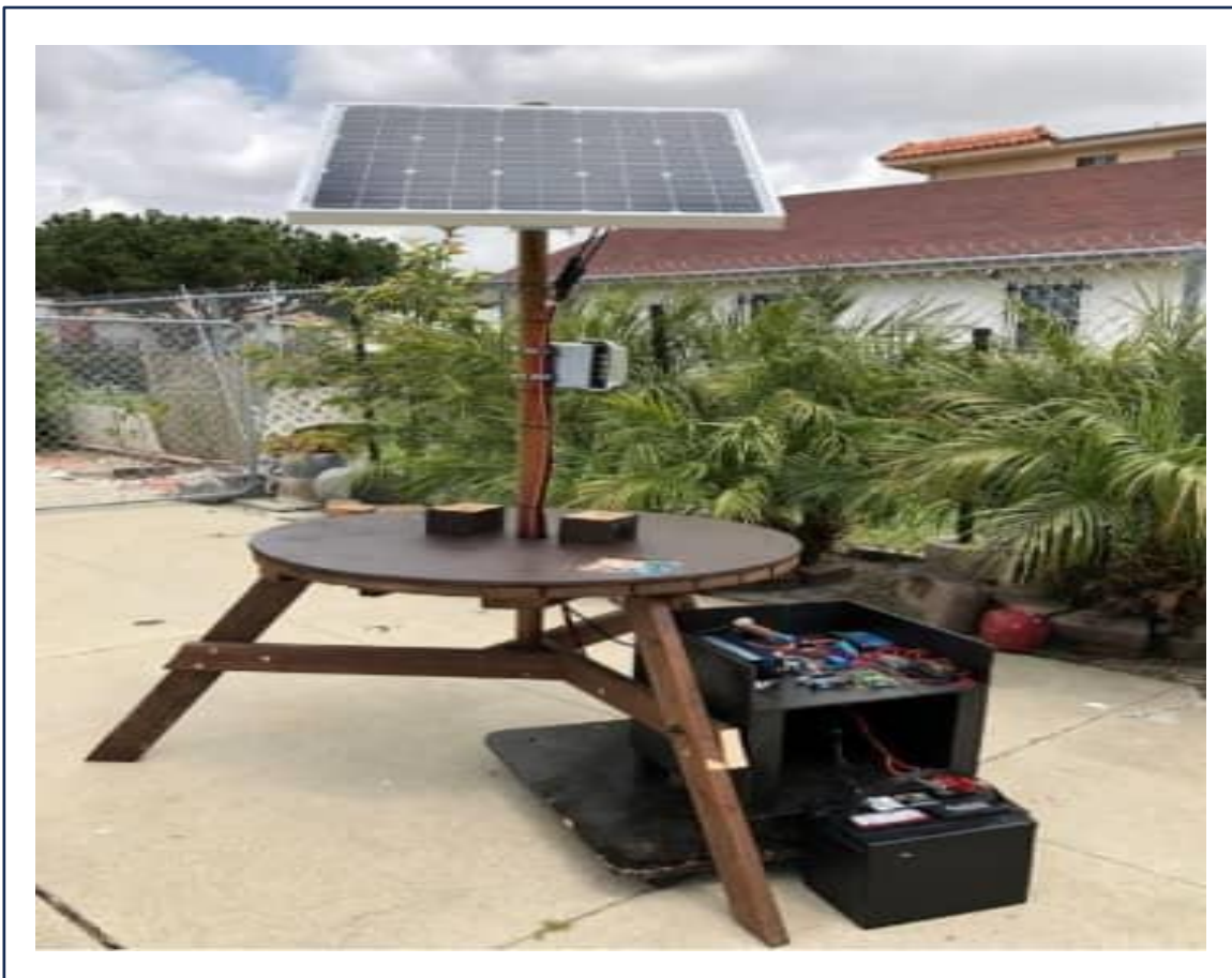
FIGURE1.8: CHARGING STATION PROTOTYPE[13]
