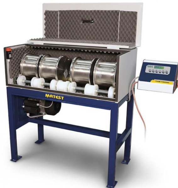
Figure II.6. The Micro Deval Machine. Ref: https://www.matest.com/fr/granulats/machines-abrasion/micro-deval-machines
