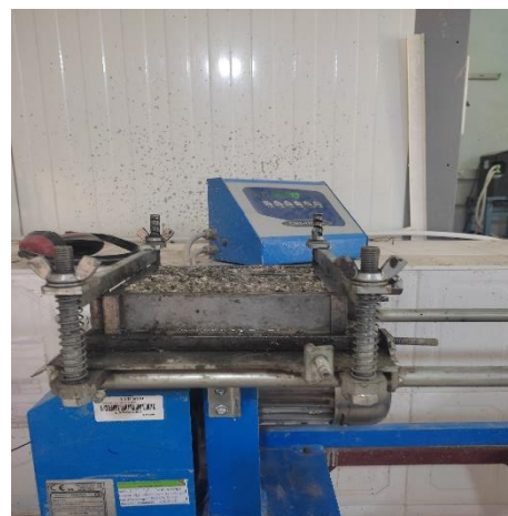
Figure II.10. Fill the mold and place it in the shock device. Ref:Author 2025
