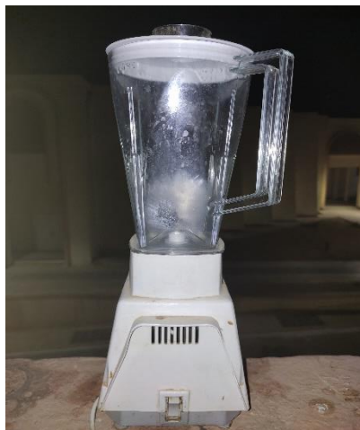
Figure II.7. Home Blender used to cut the polystyrene. Ref:Author 2025
