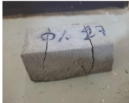
Figure II.14. Compression test carried out on the specimens (04x04x16) cm. Ref:Author 2025
