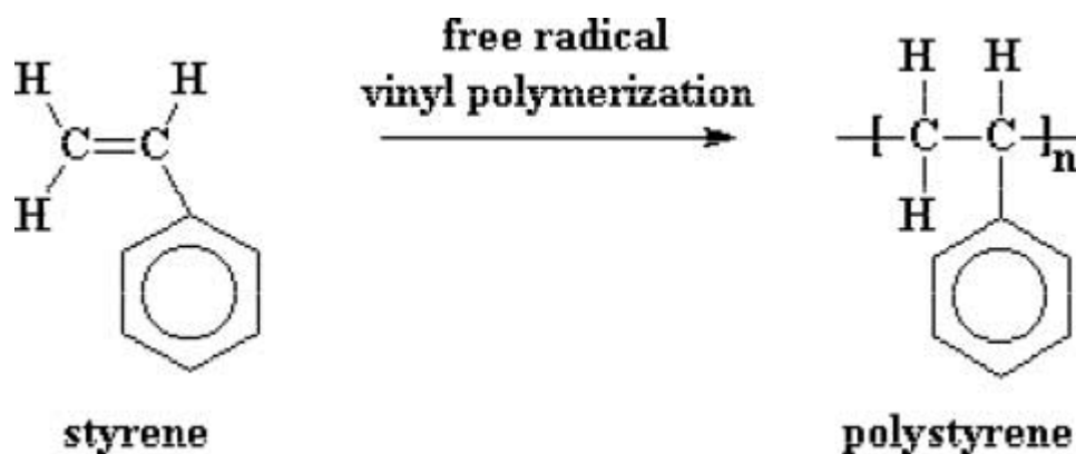
Figure.I.11.Polymerization of styrene monomer into polystyrene.
