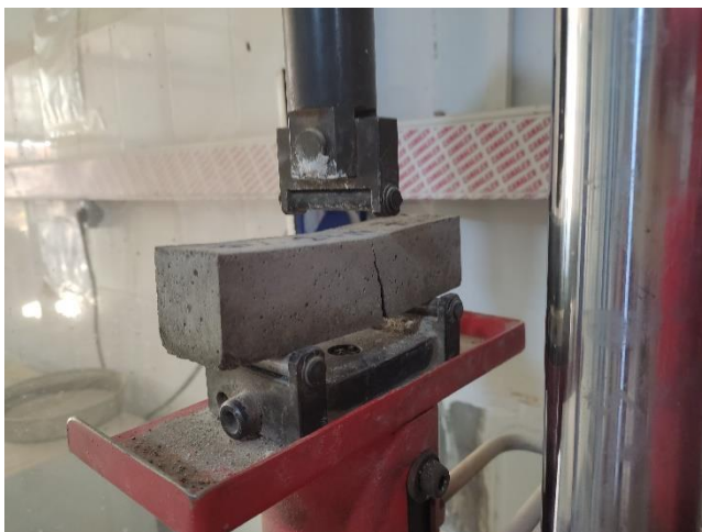
Figure II.12. Flexural failure mechanical test setup. Ref:Author 2025
