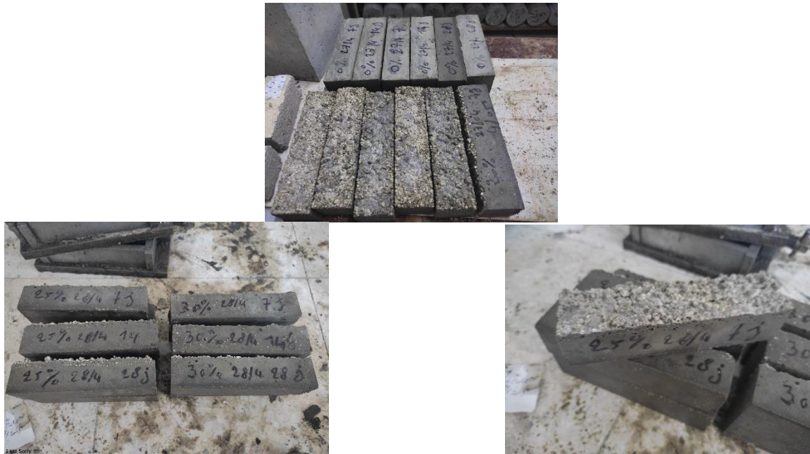
Figure II.11. Demolding and Naming the test pieces to store in the humid chamber. Ref:Author 2025
