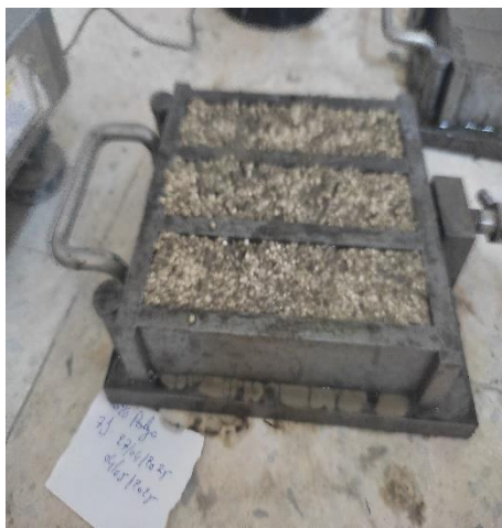
Figure II.10. Fill the mold and place it in the shock device. Ref:Author 2025
