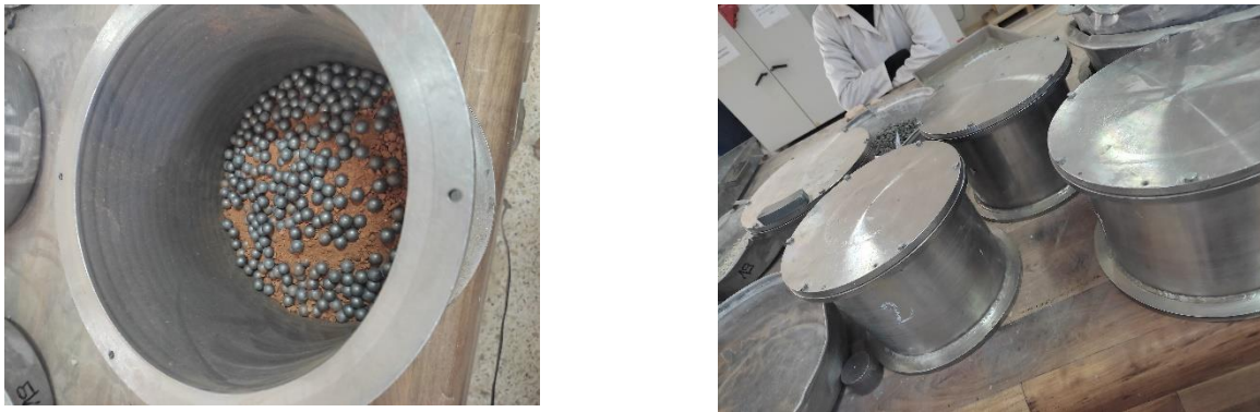
Figure II.5. Brick pellets in the mold of the Micro Deval machine with iron pellets. Ref: Author 2025
