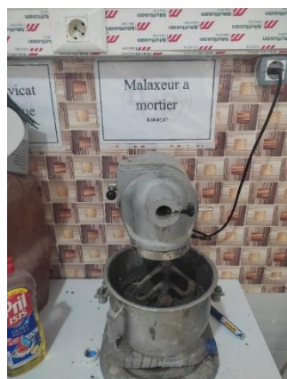
Figure II.8. Electric mixer used in mortar manufacturing [LTPS-Gardaia]. Ref:Author 2025
