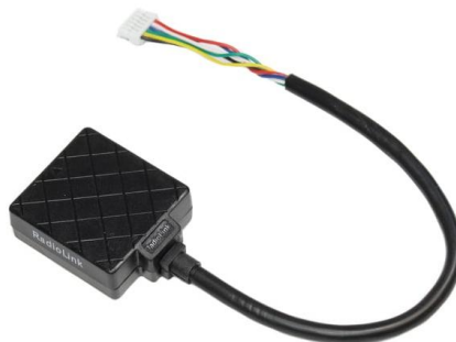
Figure VI.9: Radiolink TS100 GPS/compass
