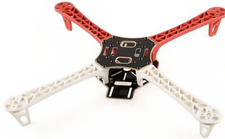
Figure VI.1: DJI F450 Quadcopter Frame
