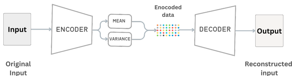
Figure 1.5—Variational Autoencoder (VAE) architecture showing input encoding to latent distribution (mean and variance), sampling, and reconstruction through the decoder.
