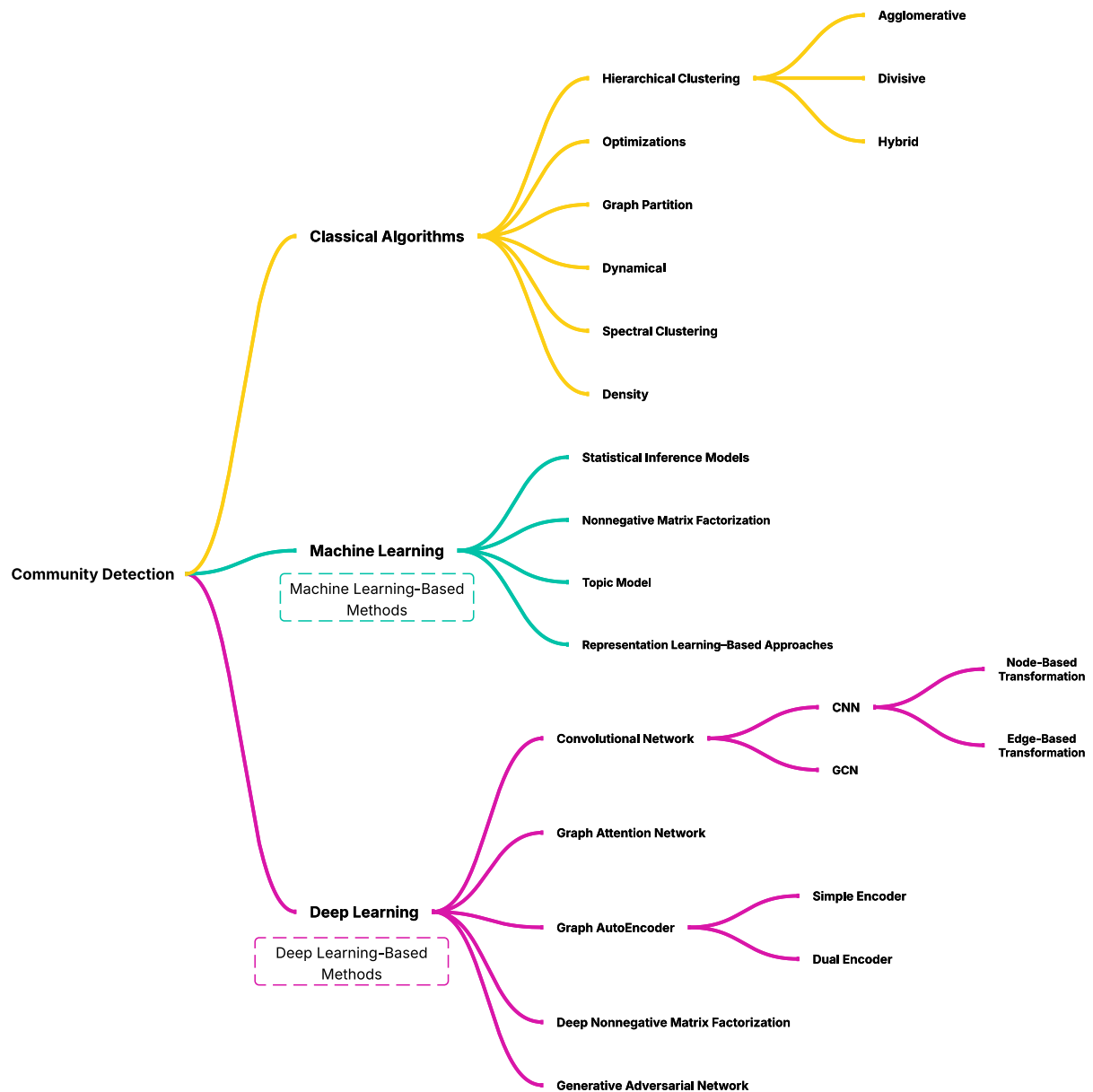
Figure 2.1—Taxonomy of community detection methods adopted in this survey. The field is organized into three main categories: classical algorithms, traditional machine learning-based approaches, and deep learning-based models. Each category contains representative techniques.
