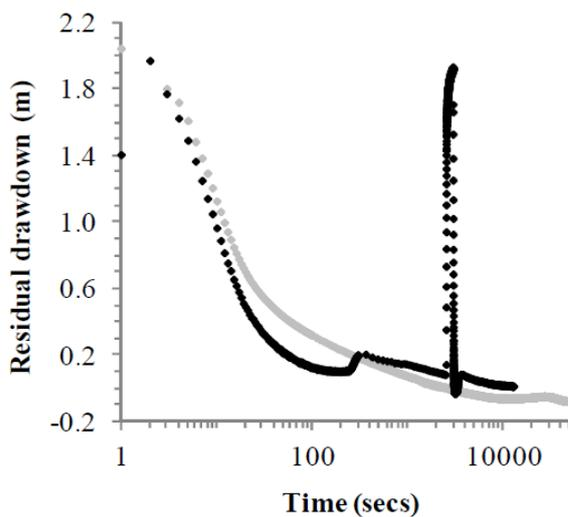
**KB 602 as an observation well during test on KB 606**
