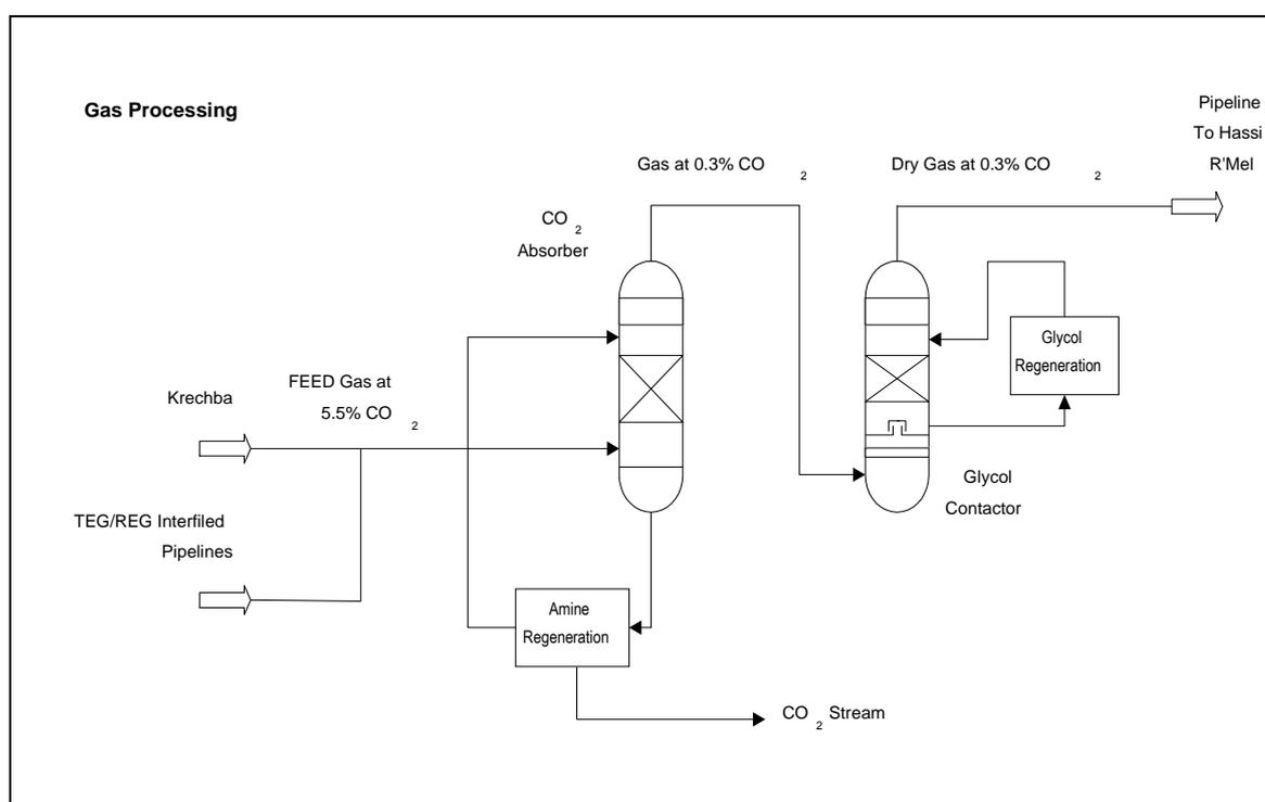
**Figure I.4: CO<sub>2</sub> Process.**
