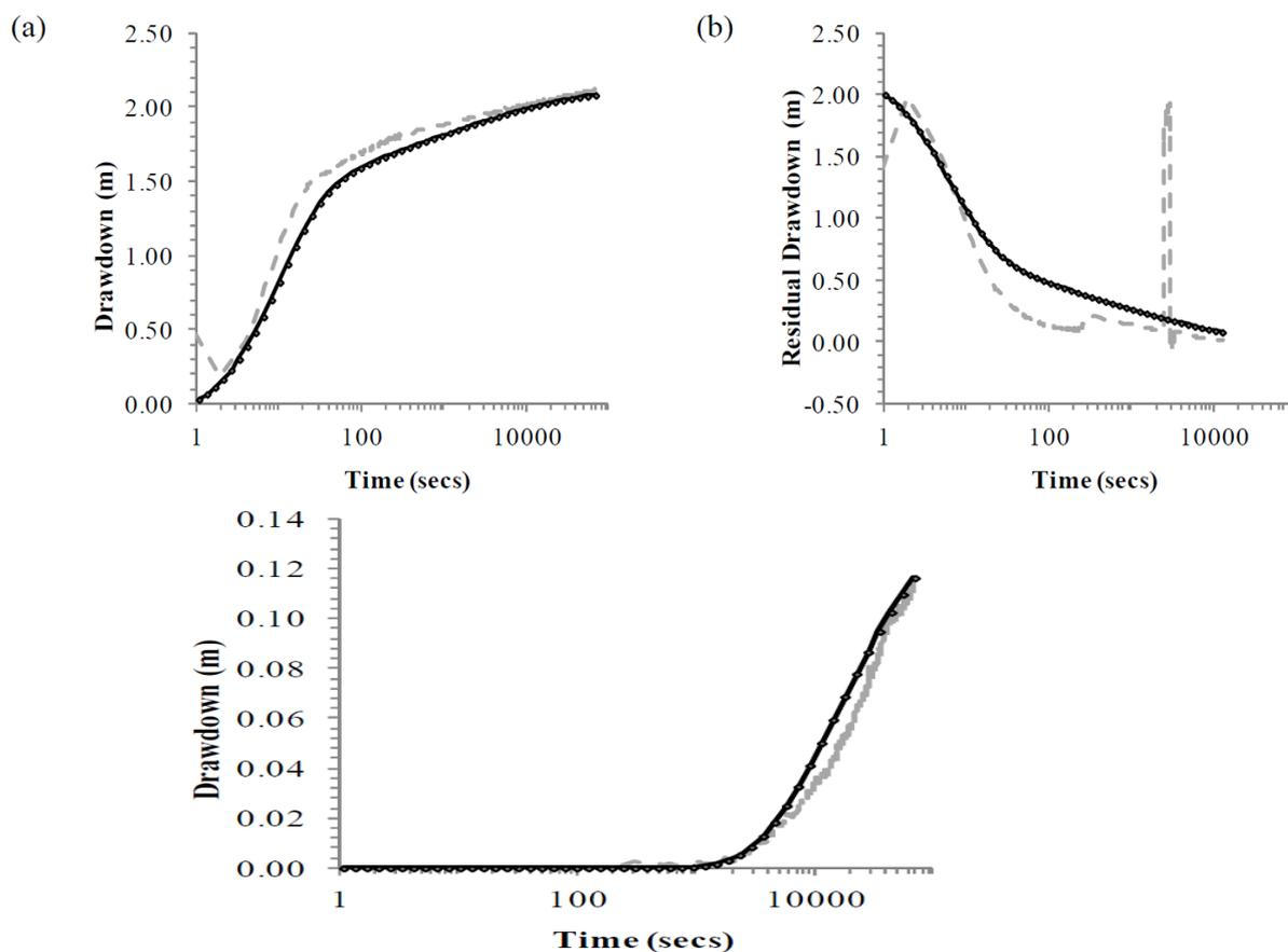
**Figure III.14. Observed (grey) and simulated (black) (a) time-drawdown recovery curves for observation well for KB 606 test**
