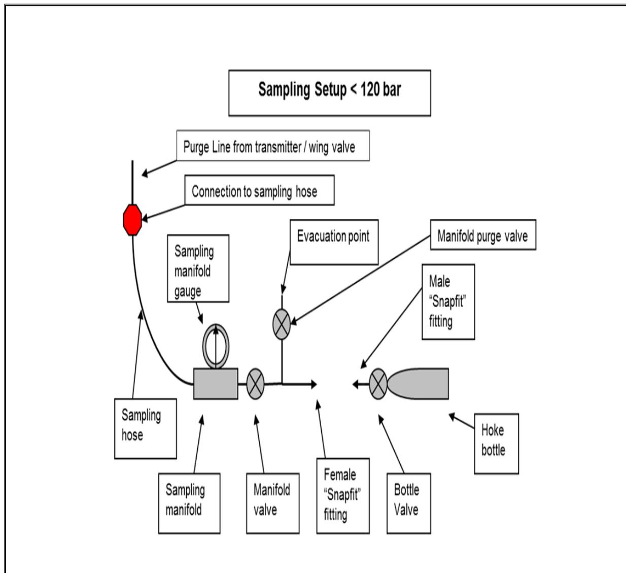
**Figure. II.12. Schematic Explains Gas Sampling method**
