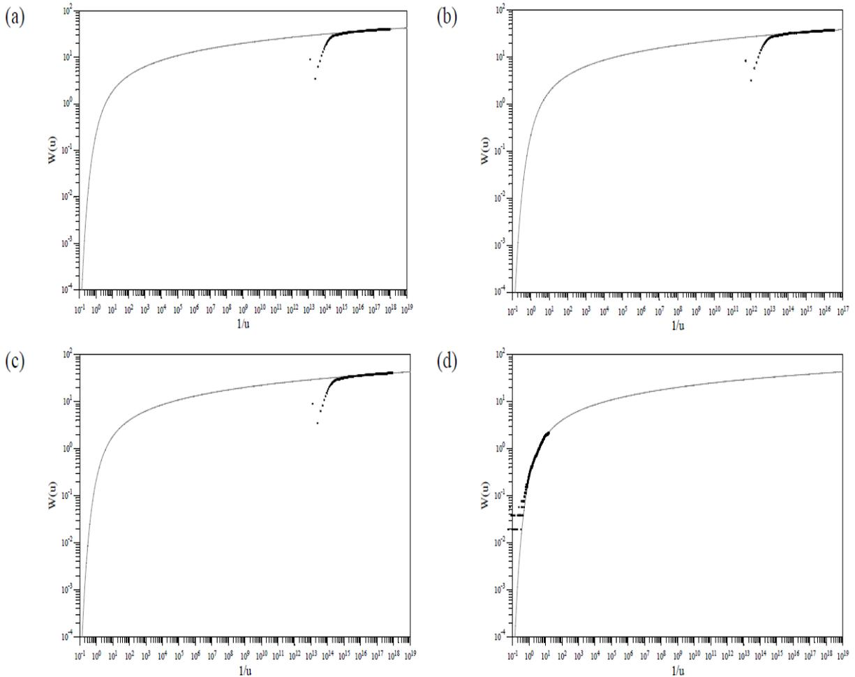
**Figure III.12.** This analysis of pumping tests at boreholes (a) KB 602, (b) KB 603, (c) KB 606 and (d) KB 602 as an observation well during test on KB 606.
