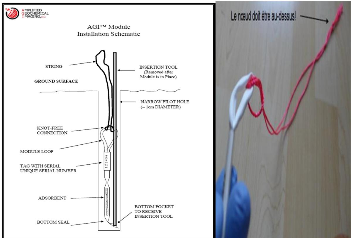
**Figure. II.10. The schematic installation module**
