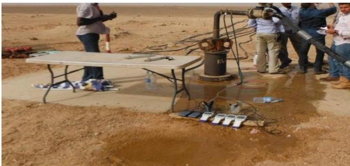
**Figure III. 9. Surface equipment setup showing borehole manifold, flow meter and sampling taps.**
