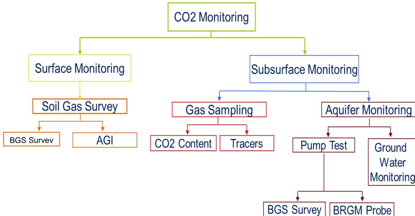
**Figure II.6: Actual technologies applied at Krechba**
