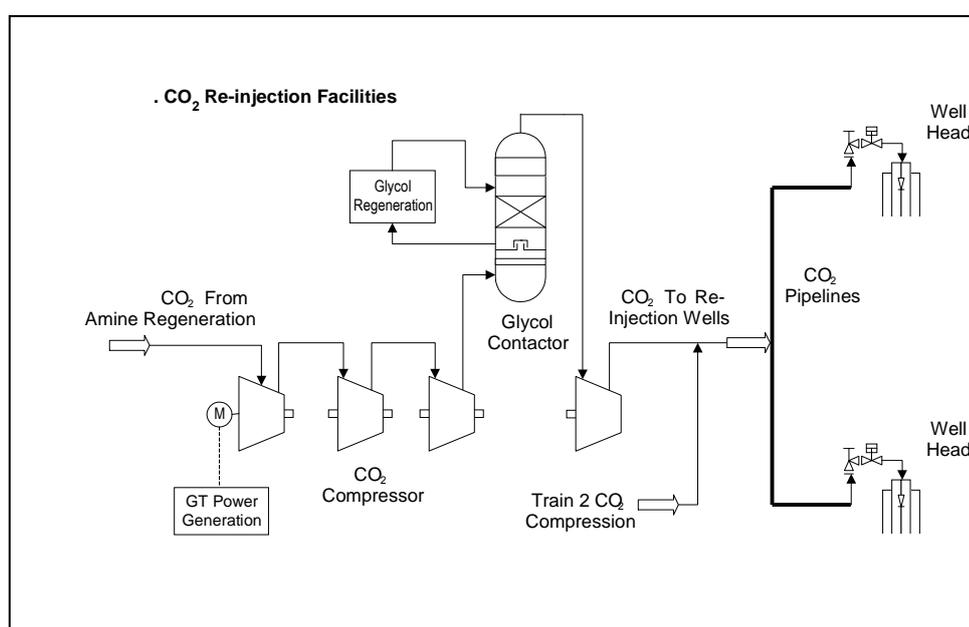
**Figure I.5: CO<sub>2</sub> Reinjections Facilities.**
