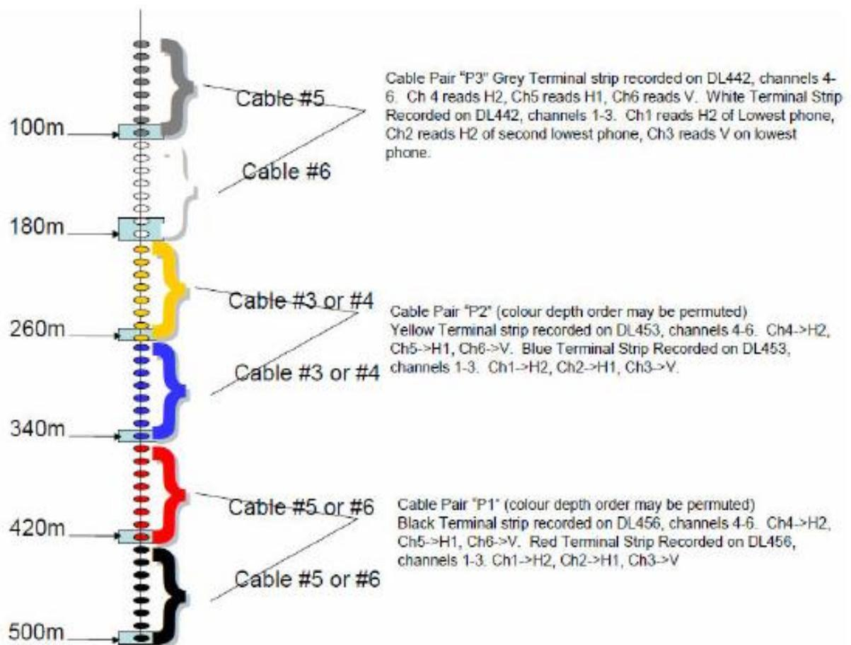
**Figure II.4: Arrangement of installed geophone array in KB-601**
