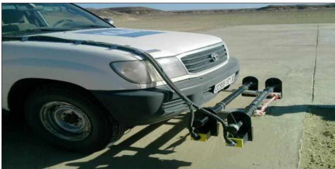
**Figure.II.7. Open-path laser CO<sub>2</sub> and CH<sub>4</sub> detectors were mounted on Toyota car**
