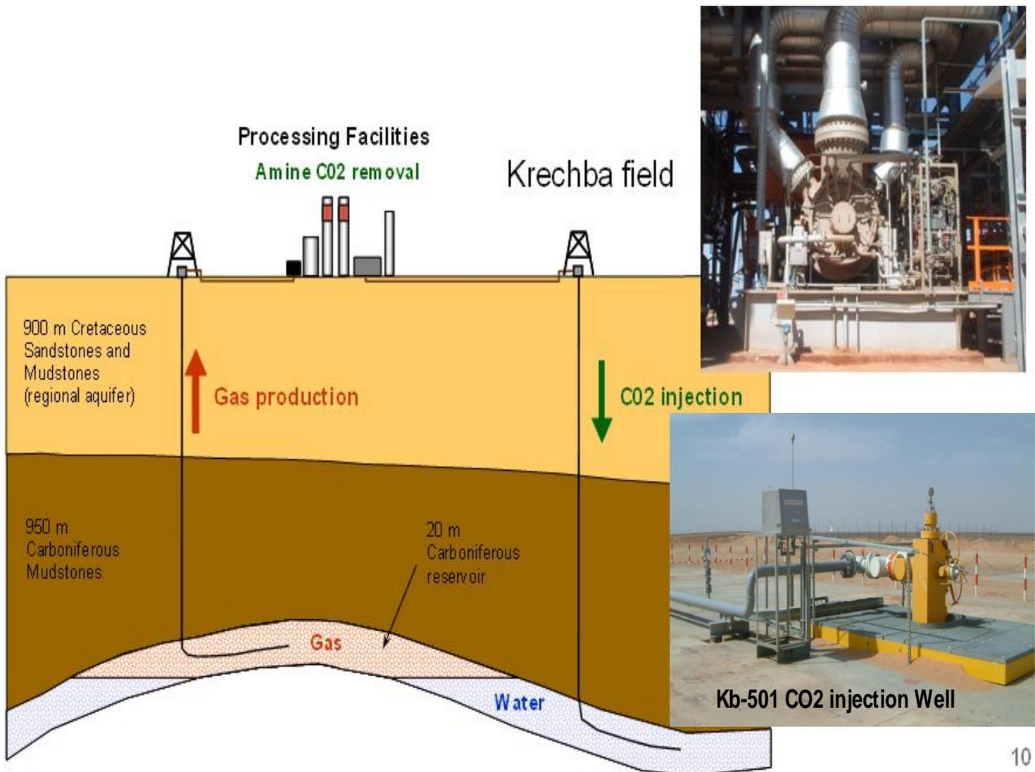
Figure I.6: Cycle of re-injection CO<sub>2</sub>.
