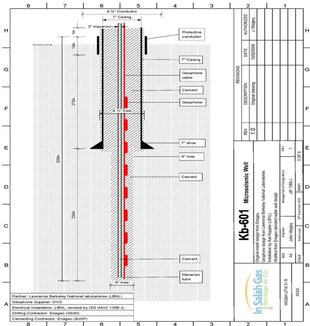
Figure II.5: well completion design in KB-601
