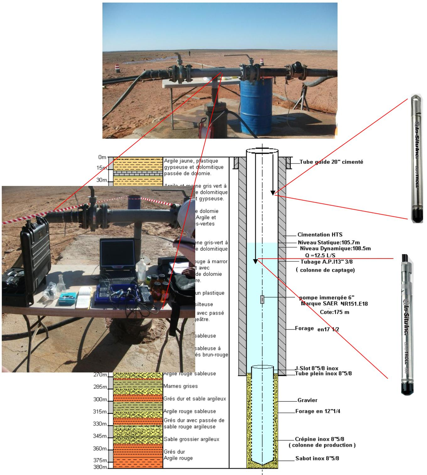
Figure III.7. Schematic showing layout and equipment for pump testing aquifer monitoring wells
