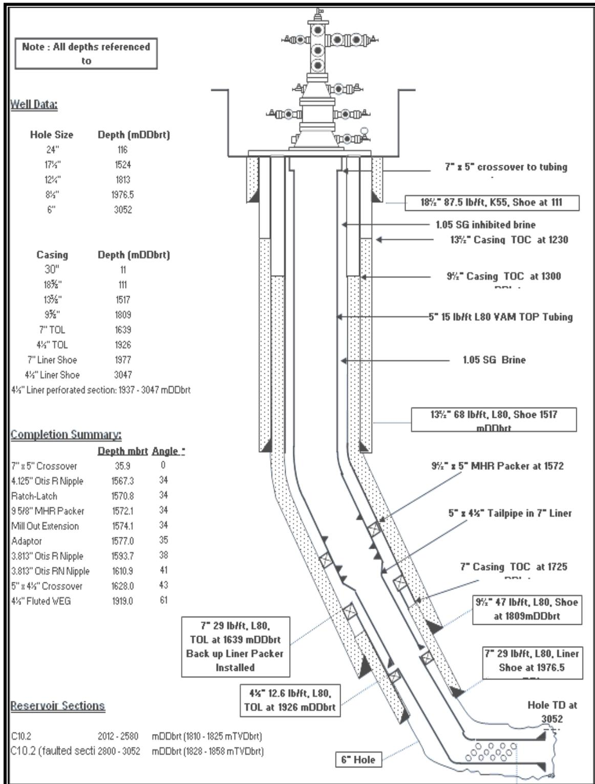
Figure.6.1 Well completion design of injector well
