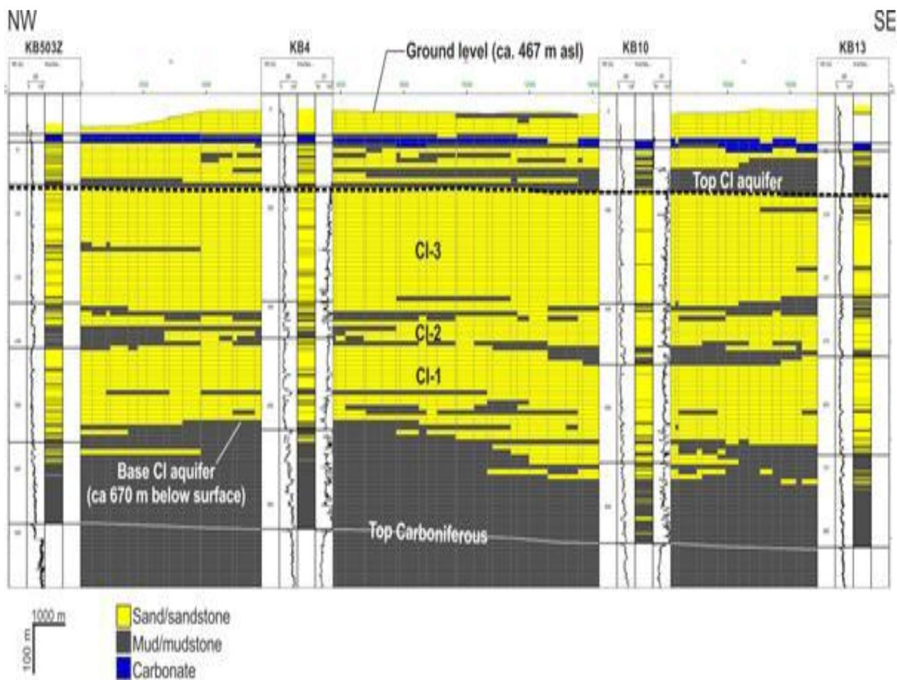
**Figure III. 4. Northwest to southeast cross-section across the Krechba site showing four wells.** Tracks for gamma-ray log, facies and sonic velocity (where available) plotted against the cellular geological model. (Asfirane et al 2012).
