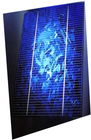
Figure I.8 : Silicium poly cristallin.
