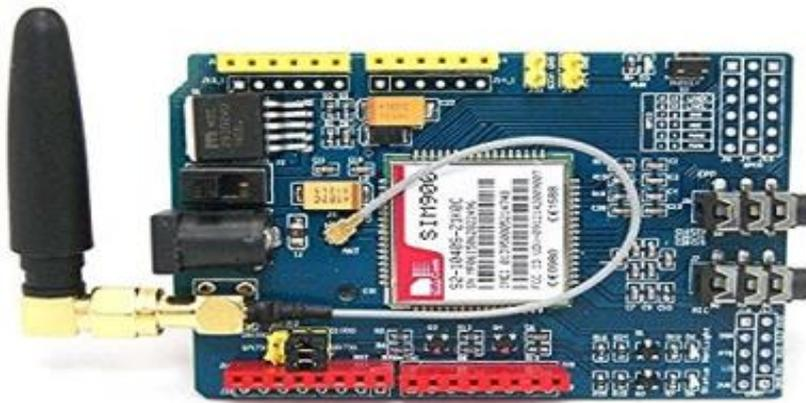
Figure II.8: module GSM SIM 900[30]
