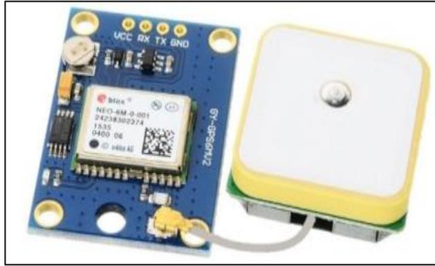
Figure II.10: Module GPS NEO-6m [32]
