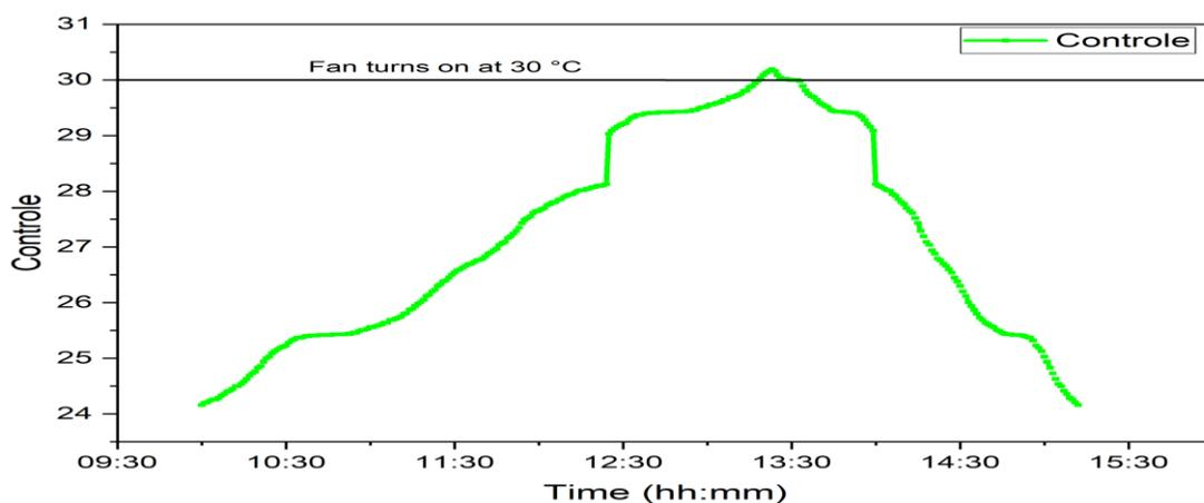
Figure (5): Temperature evolution in a greenhouse with control
