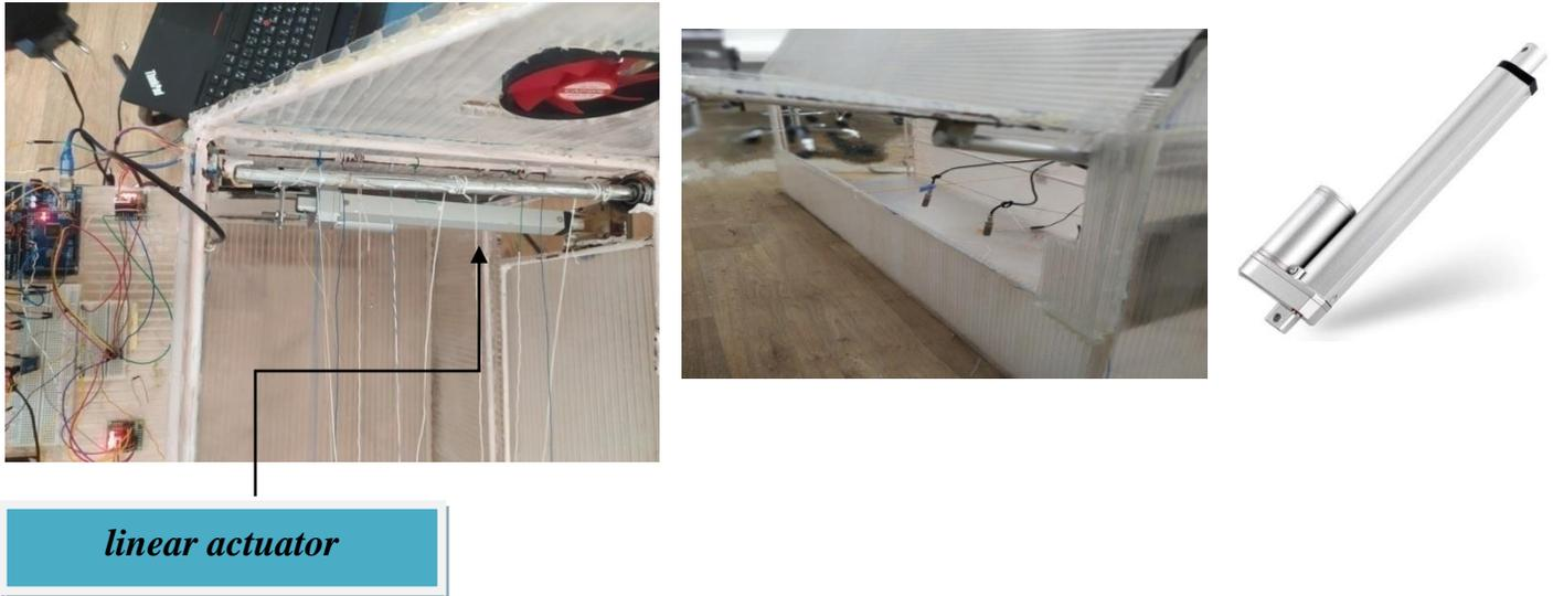
Figure III.3.4: Operating of natural ventilation system
