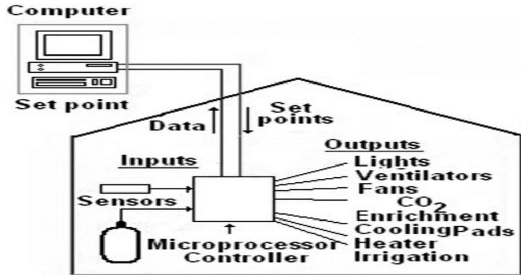
Figure I.8.1 : Computerized Control Systems in Greenhouse.
