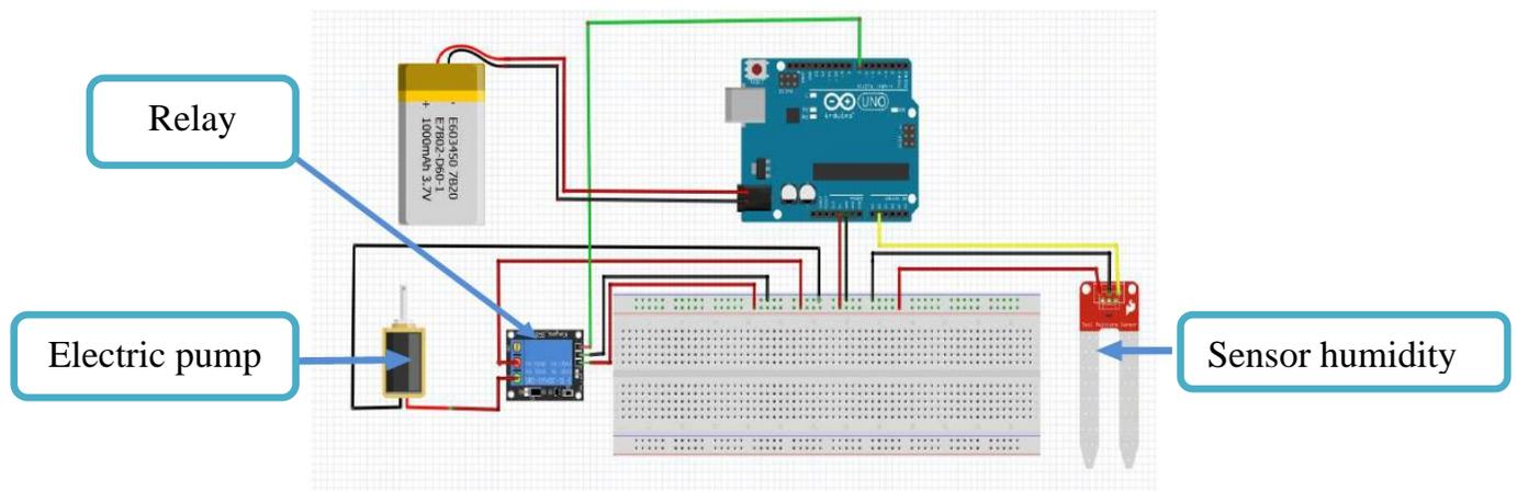
FigureIII.3.2: Mounting the soil moisture sensor.
