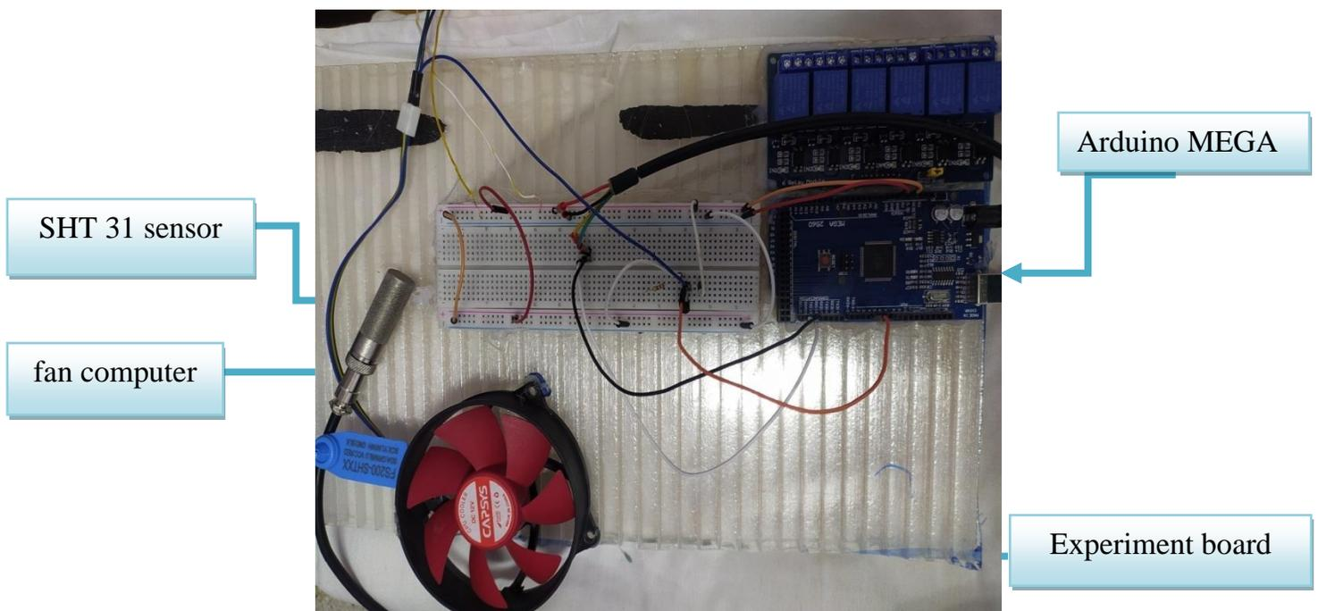
Figure III.3.2: Mounting the **SHT 31** sensor
