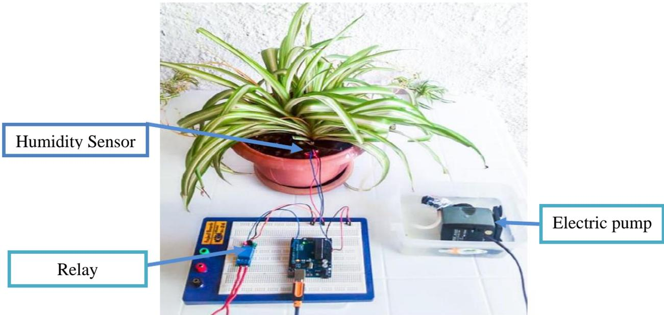
Figure III.3.1: Mounting the soil moisture sensor.
