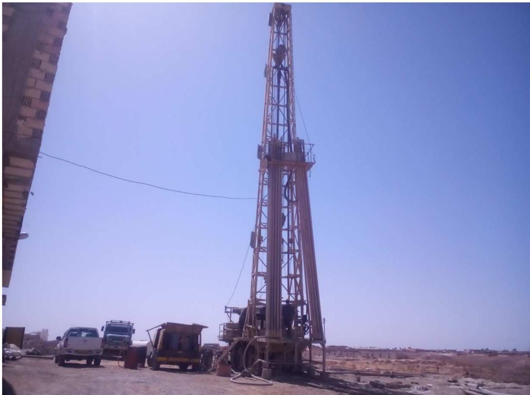
Appareil ROTARY de type SPEED START 35 (ss-35)
