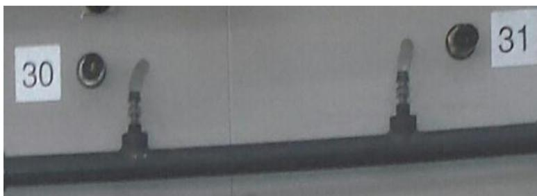
**Figure 17 : (30,31) rugueux conduite (Ø17mm – Ø14mm)**
