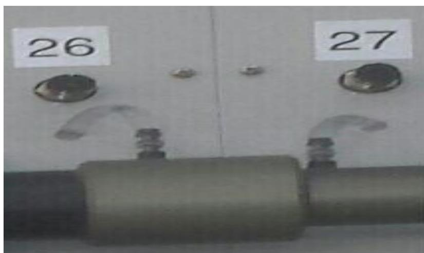
**Figure 13 : (26,27) expansion (Ø26mm – Ø52mm)**
