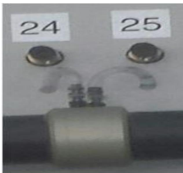
**Figure 14 : (24,25) orifice (Ø20mm)**
