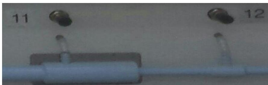
**Figure 22 : (11,12) soudaine contraction (Ø26,2mm – Ø13,6mm)**
