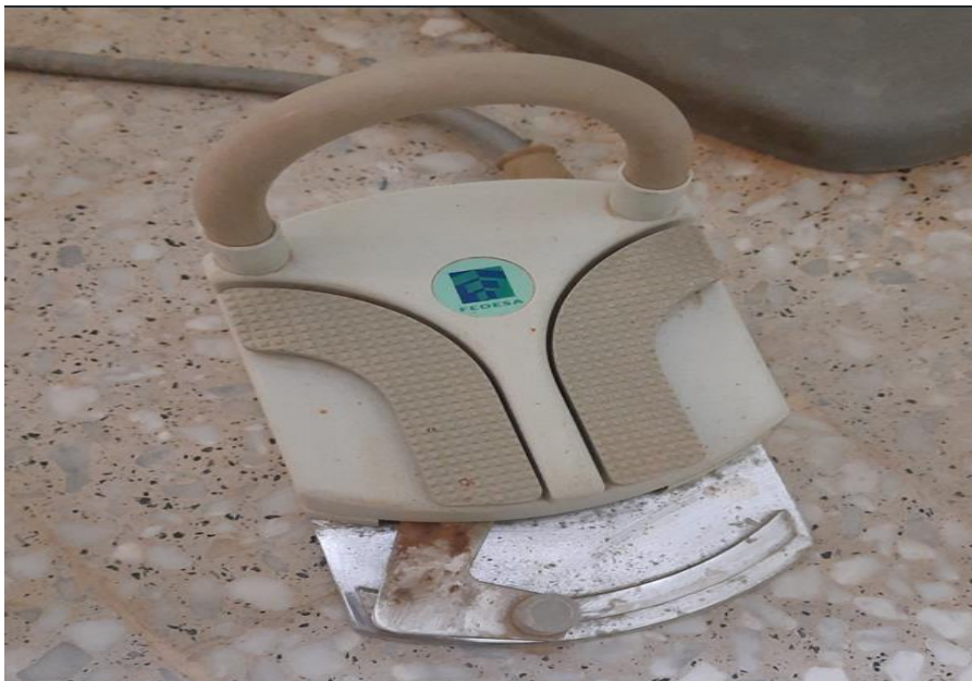
Figure 1.8: Pneumatic foot pedal
