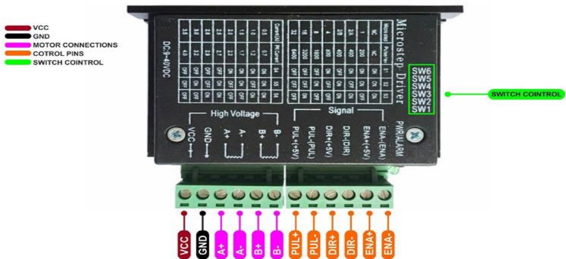
Figure 3.1: TB6600 Stepper Motor Driver Module
