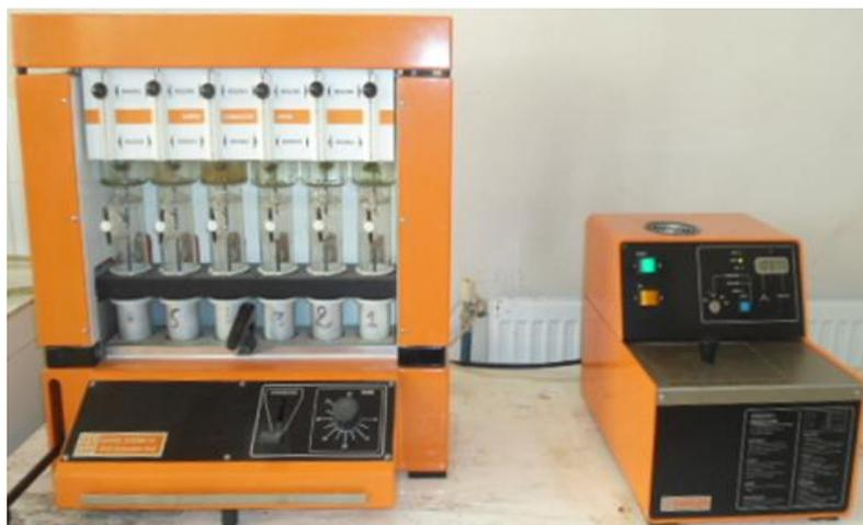
**Figure 06 : Appareil Soxhlet (Djouza, 2014)**
